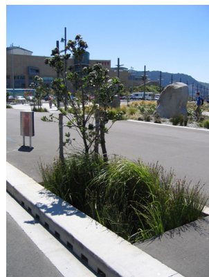
Street tree bioretention systems to treat runoff from Porter Street equating to approx. 30m 2 of bioretention area to be provided. The final number of trees will be dependant on available space and position of existing trees.
