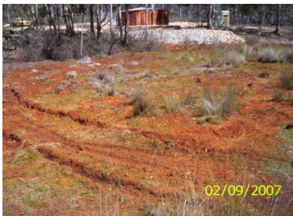
Photo 1 & 2: Iron & Manganese deposits - Invincible Colliery Drainage Borehole, Ben Bullen SF
