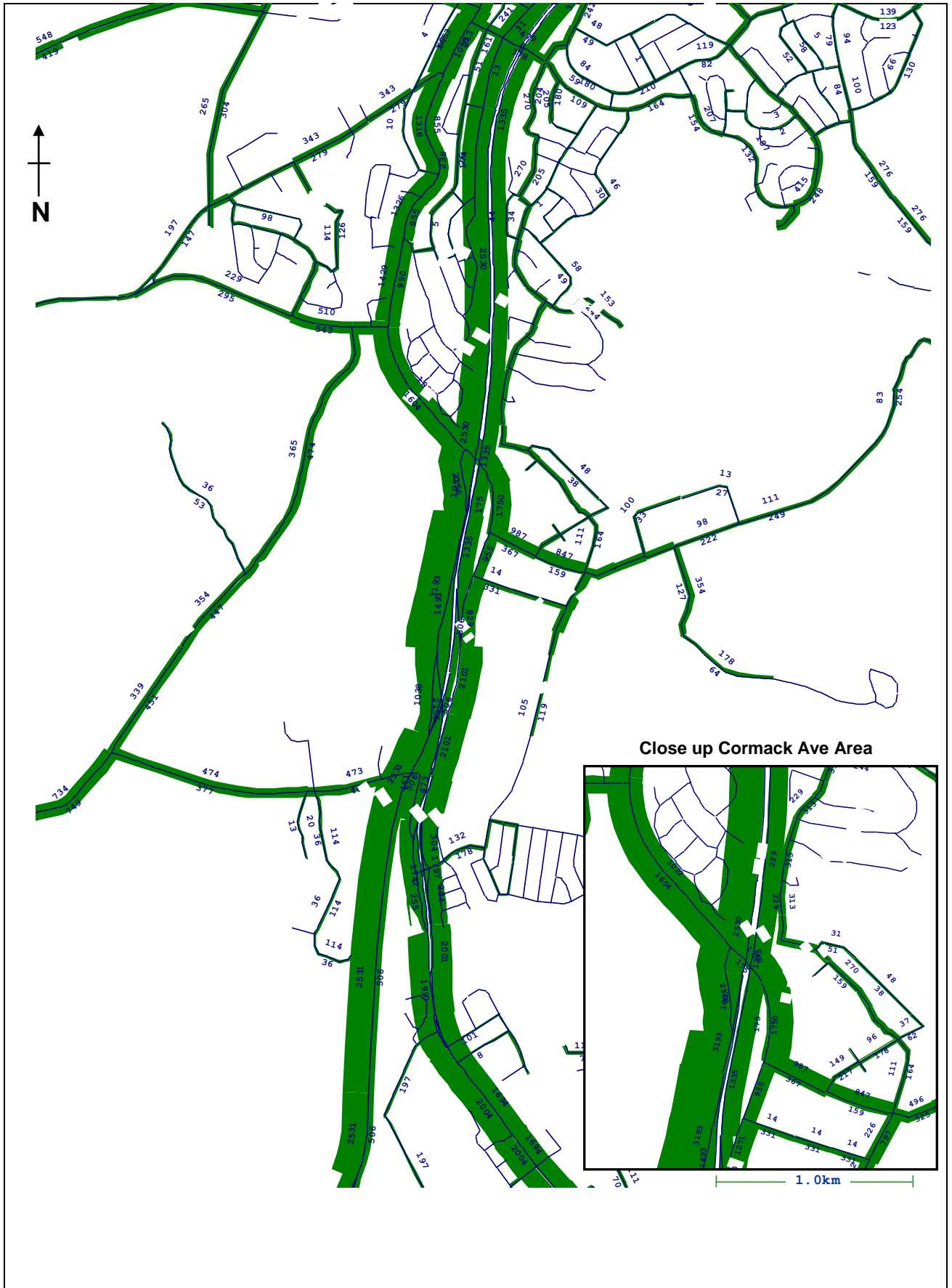
Tallawarra Transportation Model 2036 No Cormack Ave Connection to Princes Highway Traffic Volume Plot AM Peak Figure 51 Gabites Porter Consultants
