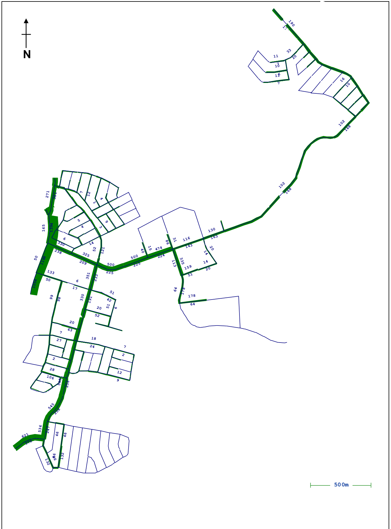
Tallawarra Transportation Model 2036 Internal Development - With Hayward's Link Traffic Volume Plot AM Peak Figure 39 Gabites Porter Consultants
