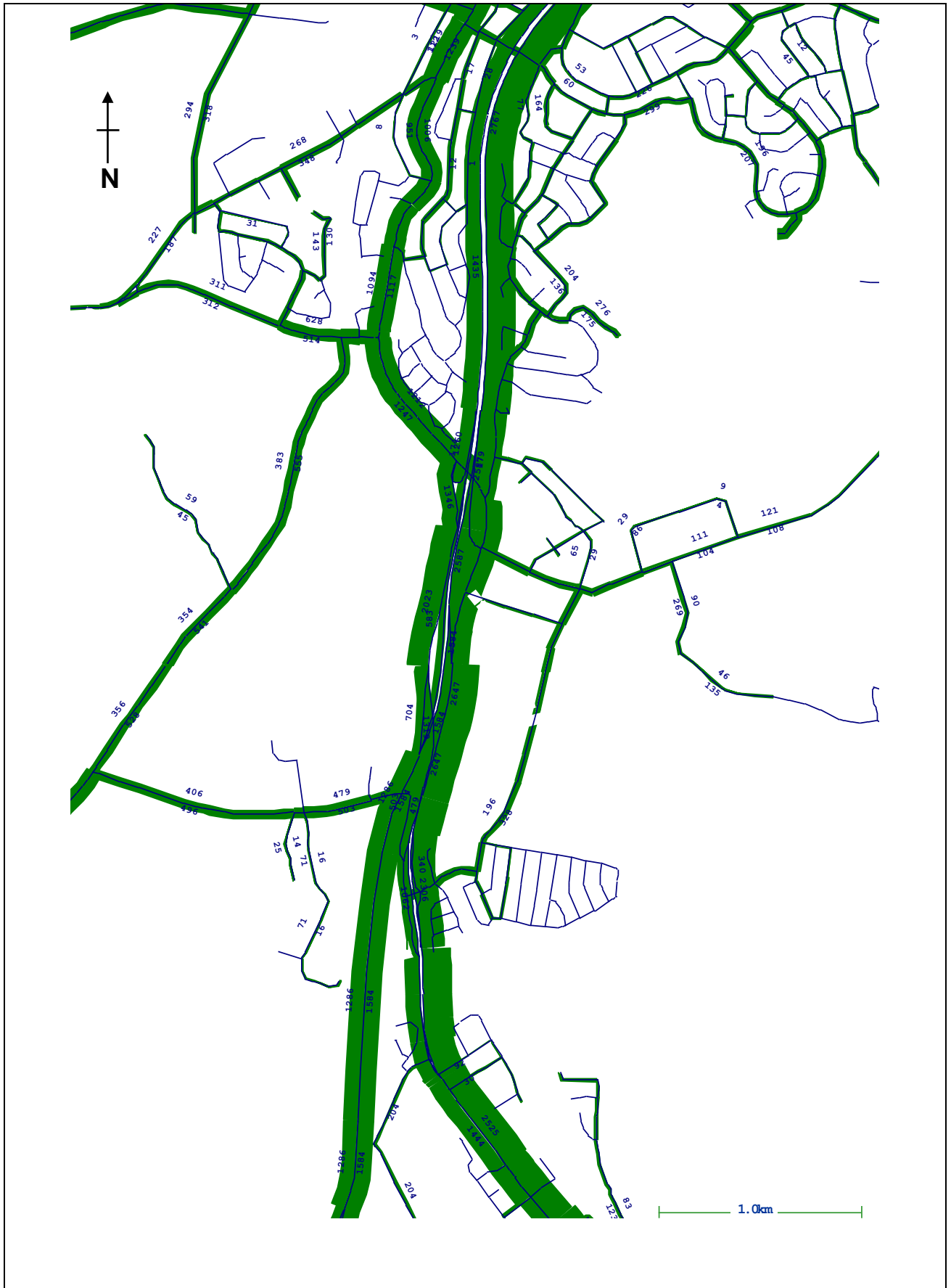
Tallawarra Transportation Model 2036 F6 Ramps + Haywards Bay Link With Tallawarra Traffic Volume Plot PM Peak Figure 58 Gabites Porter Consultants
