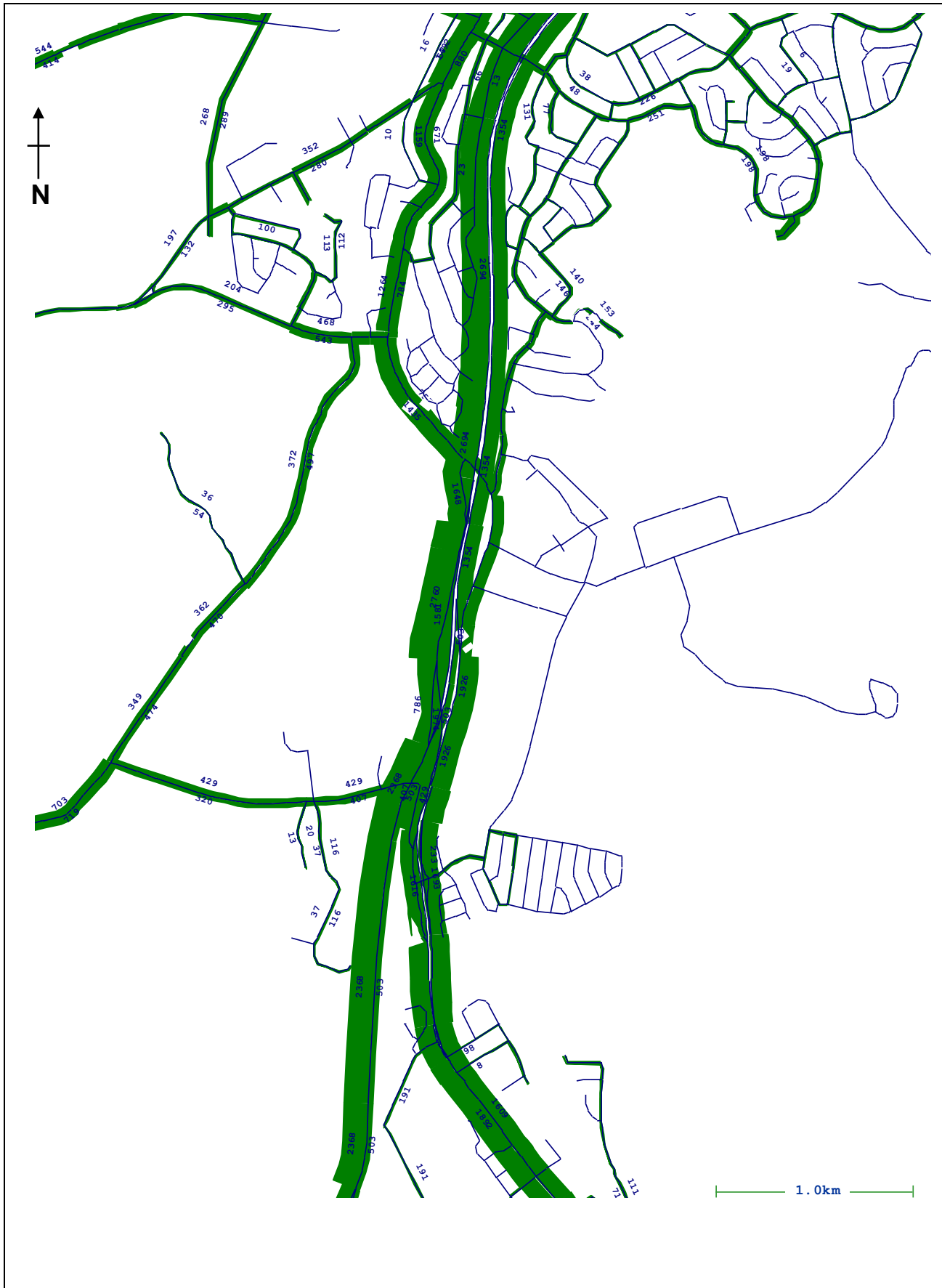
Tallawarra Transportation Model 2036 No Tallawarra Development Traffic Volume Plot AM Peak Figure 3 Gabites Porter Consultants
