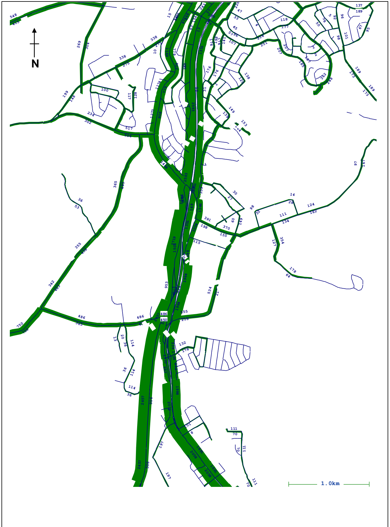
Tallawarra Transportation Model 2036 Yallah Rd Link Traffic Volume Plot AM Peak Figure 47 Gabites Porter Consultants
