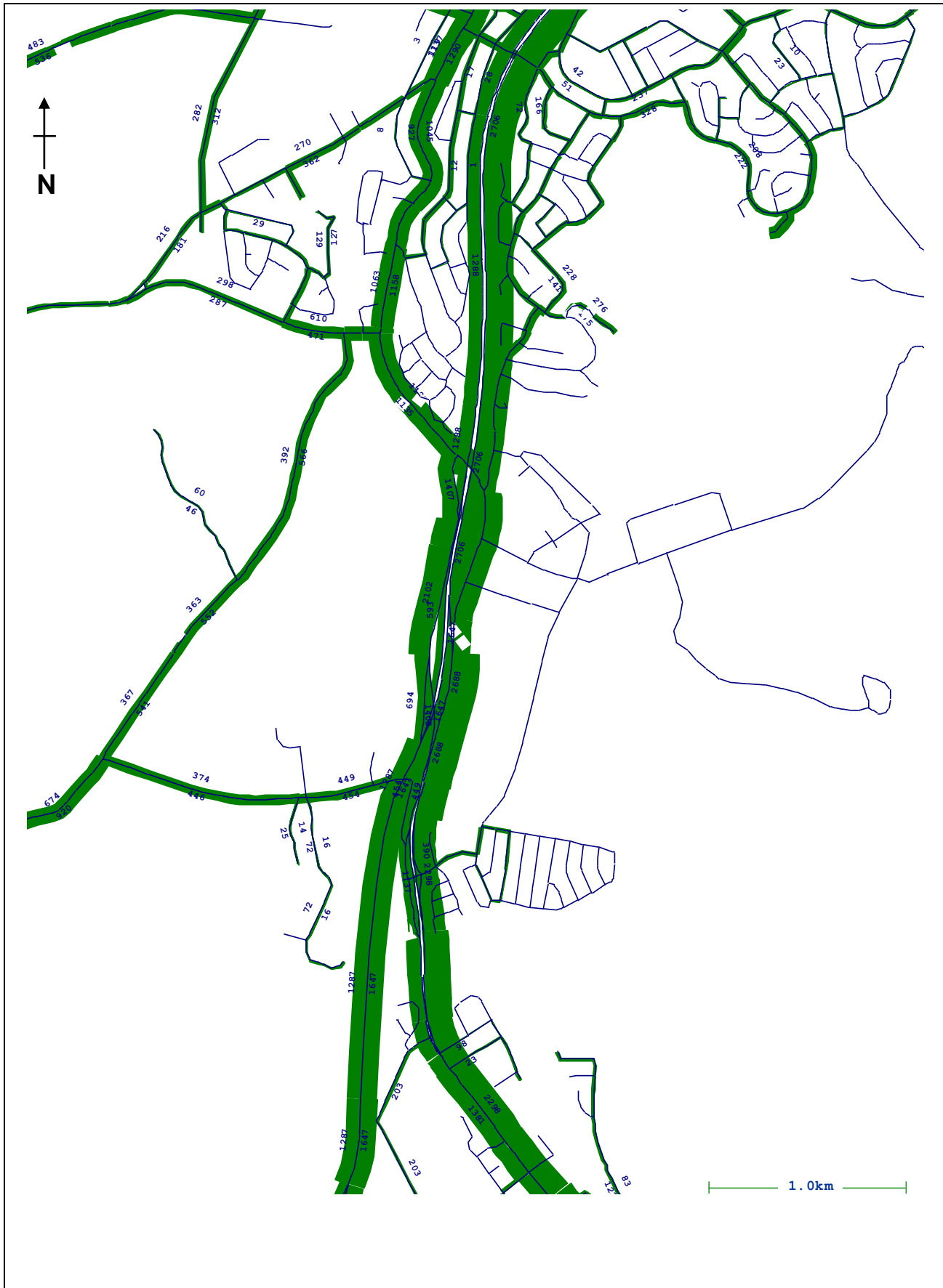
Tallawarra Transportation Model 2036 No Tallawarra Development Traffic Volume Plot PM Peak Figure 4 Gabites Porter Consultants
