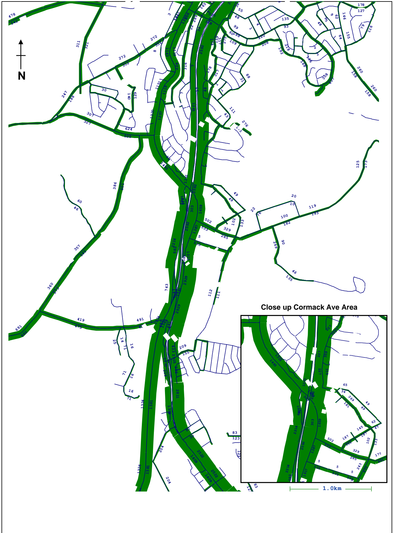
Tallawarra Transportation Model 2036 No Cormack Ave Connection to Princes Highway Traffic Volume Plot PM Peak Figure 52 Gabites Porter Consultants
