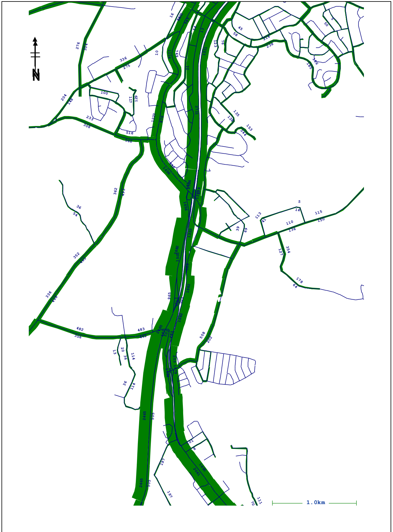
Tallawarra Transportation Model 2036 F6 Ramps + Haywards Bay Link With Tallawarra Traffic Volume Plot AM Peak Figure 56 Gabites Porter Consultants
