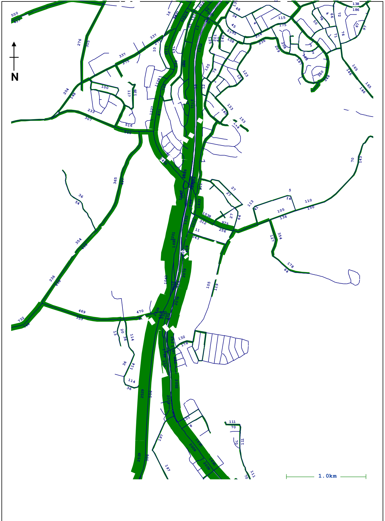
Tallawarra Transportation Model 2036 Base Without Hayward's Link With Ramps Traffic Volume Plot AM Peak Figure 27 Gabites Porter Consultants
