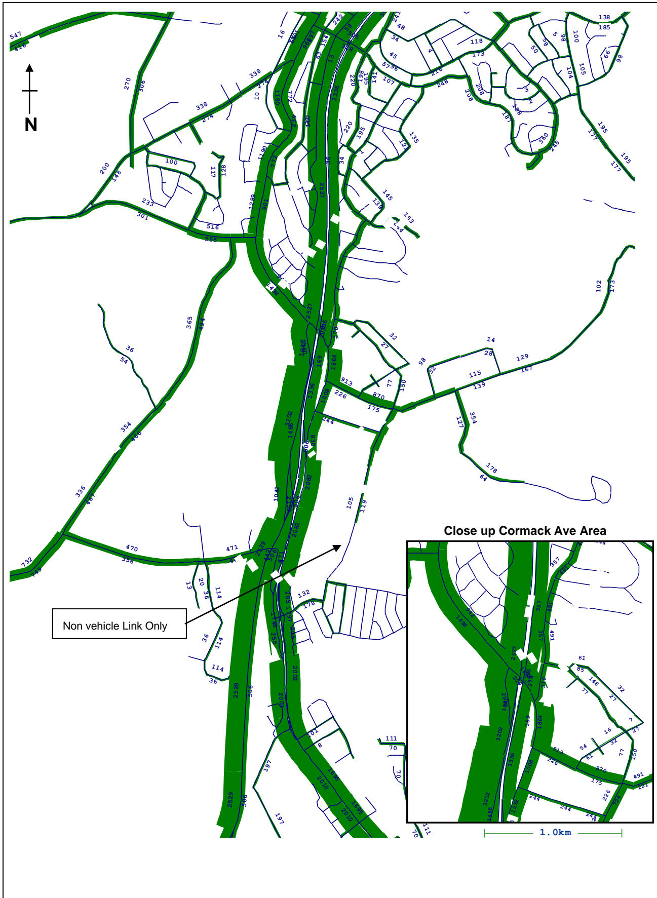
Tallawarra Transportation Model 2036 Base (No Hayward's Link) with 2 lane Princes Hwy Traffic Volume Plot AM Peak Figure 7 Gabites Porter Consultants
