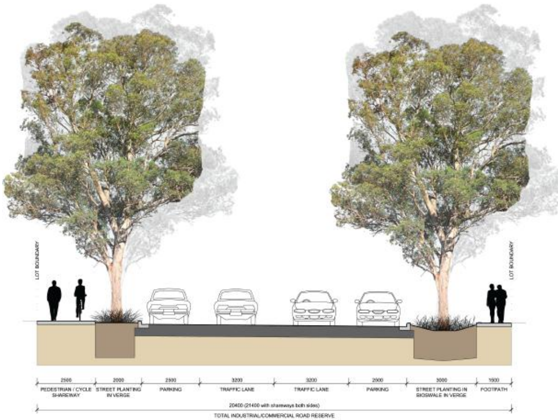
SECTION – INDUSTRIAL / COMMERCIAL ROAD WITH BIOSWALES
