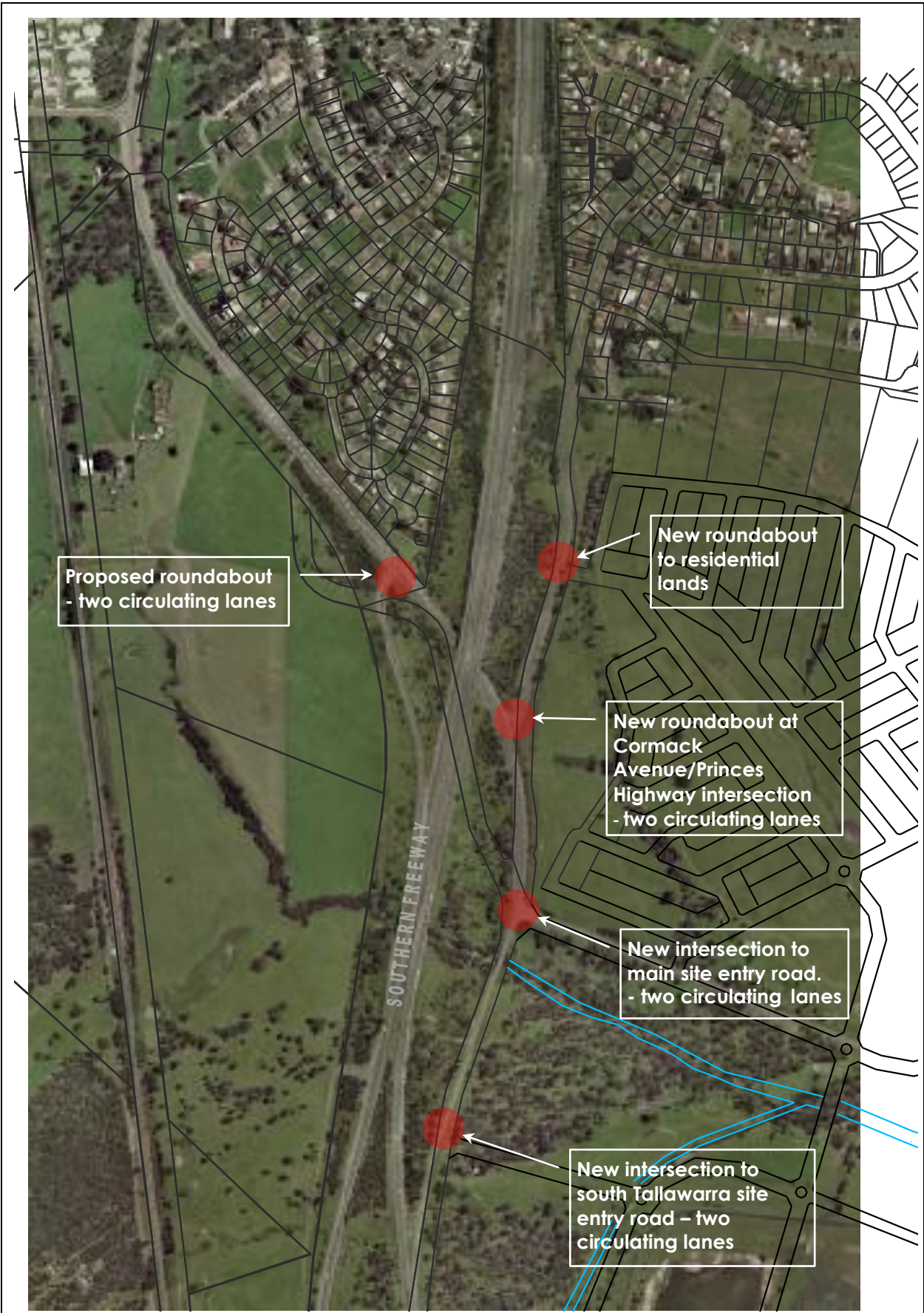
Tallawarra Lands Network Improvements required as result of Tallawarra Figure 29 Gabites Porter
