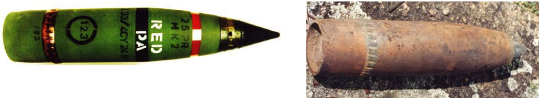
25 pdr smoke base ejection fuzed point detonating (PD) No 221 (left) and UXO (partial function) (right).
