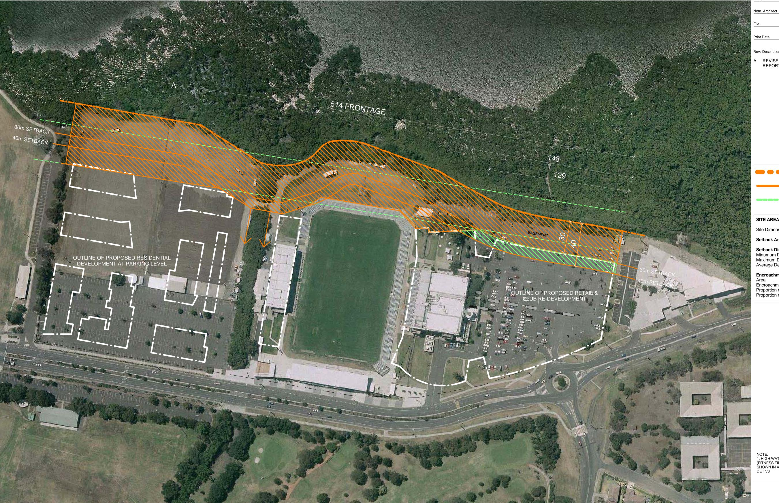
REVISED SUPPLEMENTARY 9/08/2012 REPORT MEAN HIGH WATER MARK SETBACK LINES POWER LINE EASEMENT SITE AREA 102 210m<sup>2</sup> Site Dimension Frontage 514m 21 337m<sup>2</sup> Setback Area **Setback Dimensions** Minumum Depth Maximum Depth 55m Average Depth 44.09m **Encroachment** 1399m² Encroachment Frontage 138.5m Proportion of Setback Area Proportion of Site Frontage 5.6% 26.9%
