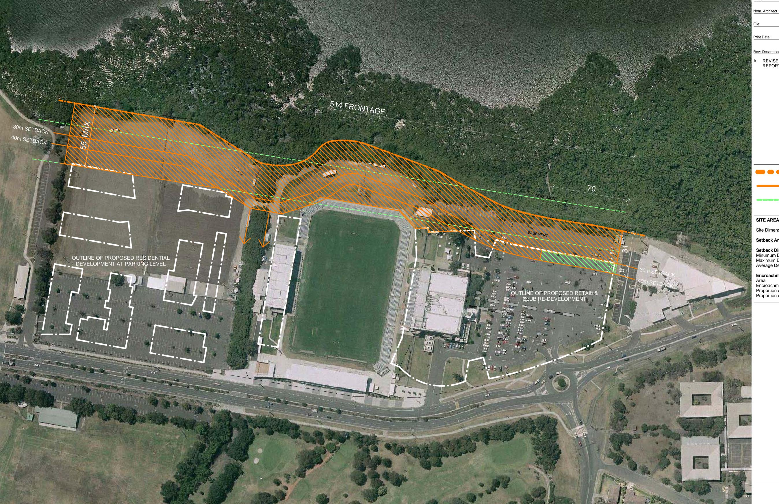
10/08/2012 4:46:06 PM Print Date: REVISED SUPPLEMENTARY 9/08/2012 REPORT MEAN HIGH WATER MARK SETBACK LINES POWER LINE EASEMENT SITE AREA 102 210m<sup>2</sup> Site Dimension Frontage 514m 24 046m<sup>2</sup> Setback Area **Setback Dimensions** Minumum Depth 31m Maximum Depth 55m Average Depth 45.64m **Encroachment** 630m<sup>2</sup> Encroachment Frontage 70m Proportion of Setback Area Proportion of Site Frontage 2.6% 13.6%
