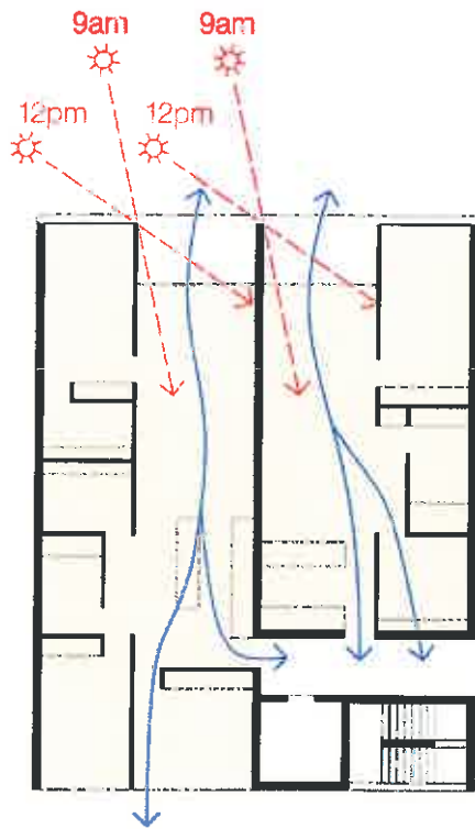
Diagram 1 Cross Ventilation and Solar Access to Typical NE Facing Units on June 21st
