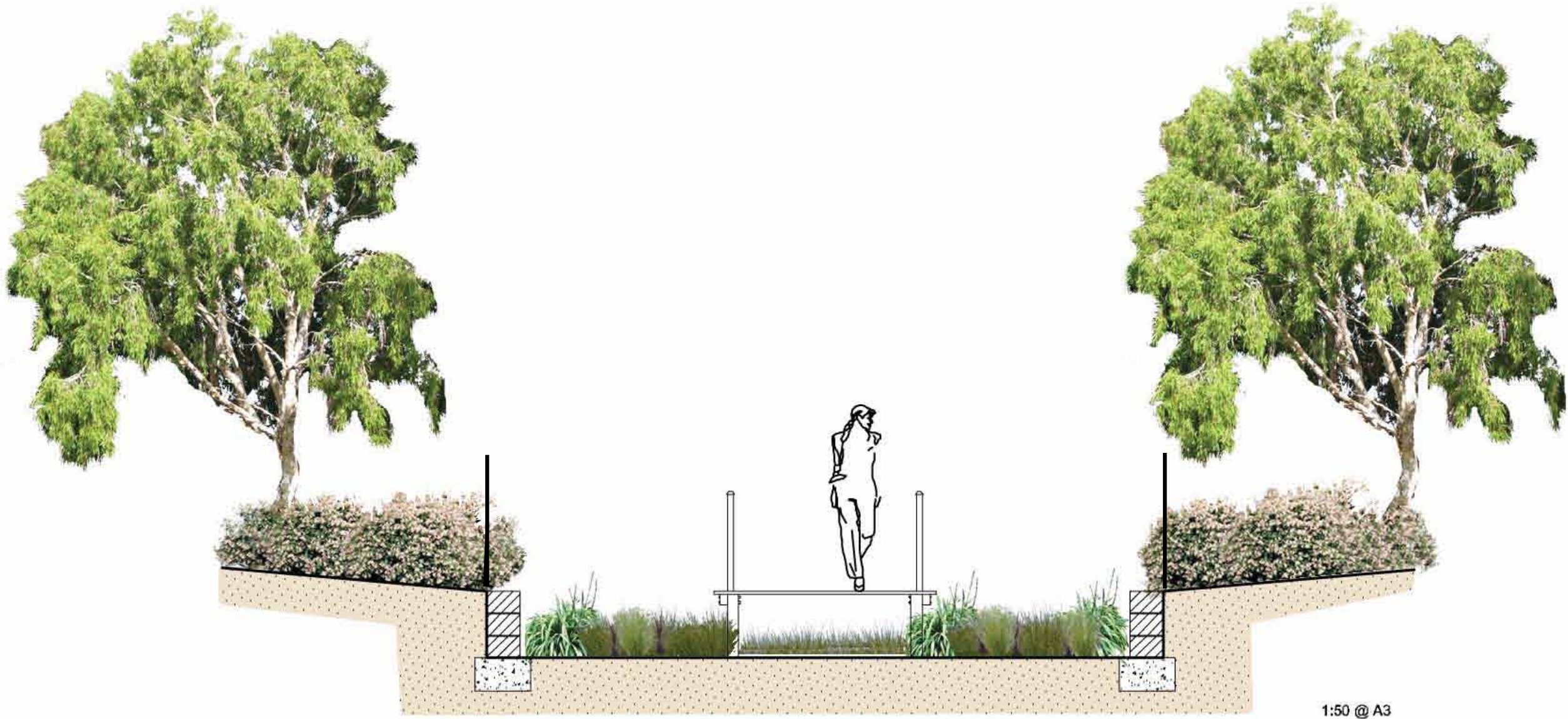
Section through Public Access Rainwater Garden
