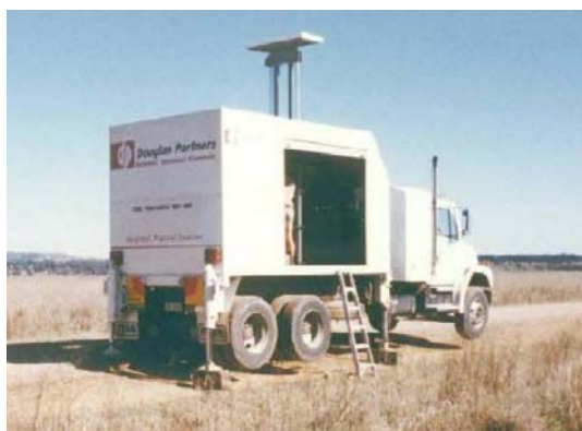
Figure 2: Purpose built CPT rig
