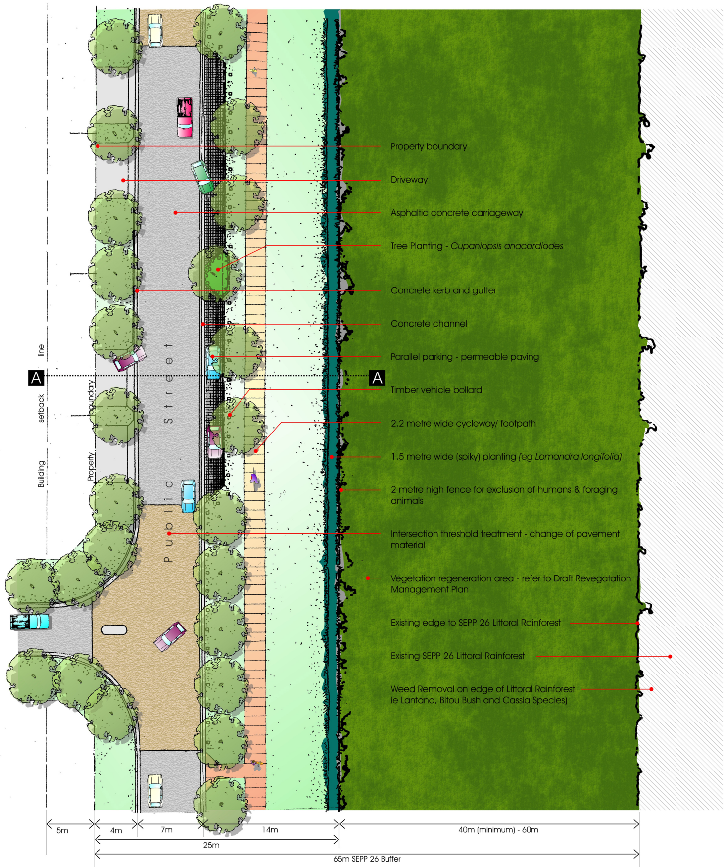
Typical Buffer to SEPP 26 Littoral Rainforest Plan Scale 1:200 @ A1
