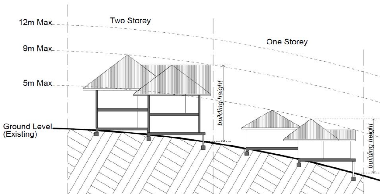
Figure 2.2.4.1 Overall Building Height
