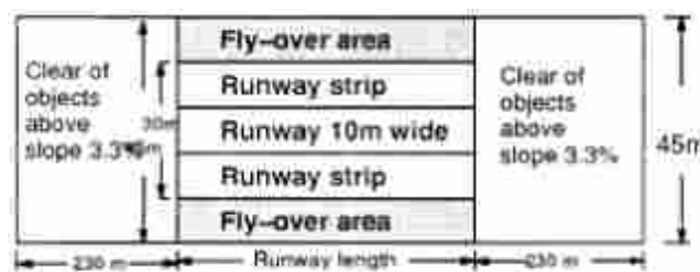
Figure 13.3 Landing ground dimensions – Agricultural Night Operations
