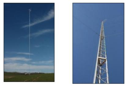
Image 4: Tubular (left) and lattice (right) wind monitoring masts Photo Courtesy: Wind Prospect CWP
