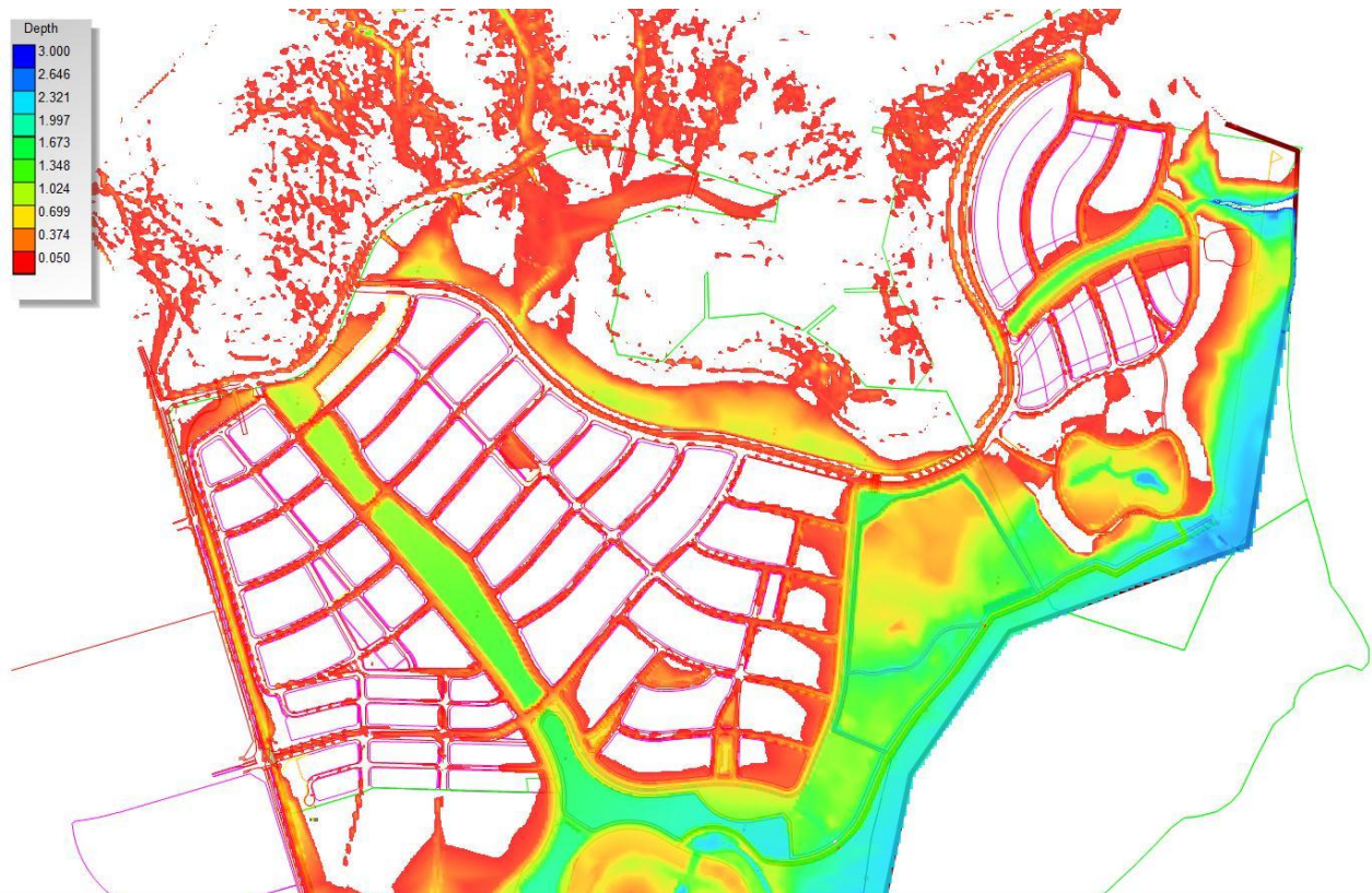
Figure E.16 – Flood Depth Mapping Across the Developed Riverside Site – 6hr 100yr Storm, Extreme Tailwater (Depth<0.05m Filtered Out)
