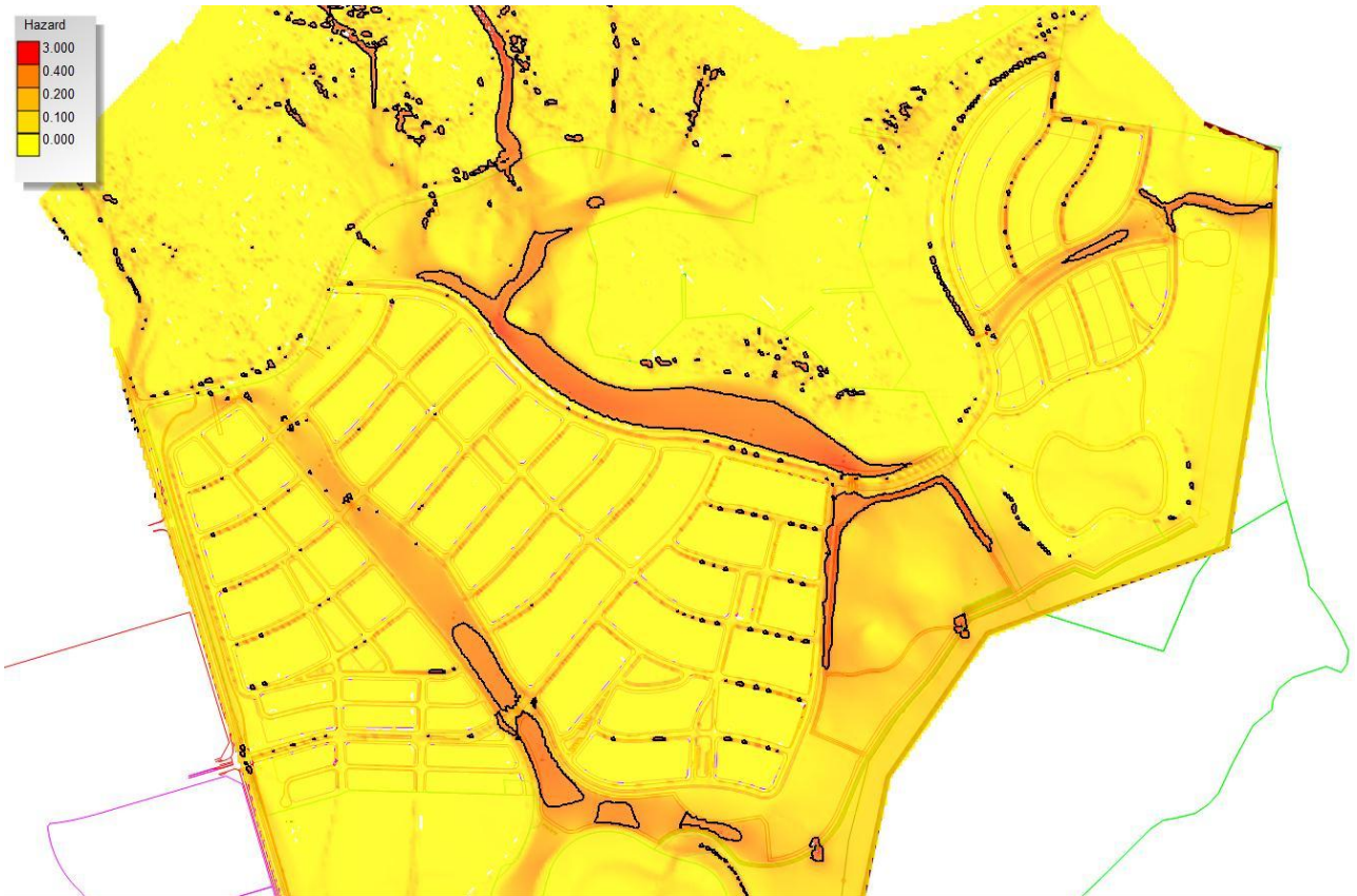
Figure E.7 – Flood Hazard Mapping Across the Developed Riverside Site – 6hr PMF Storm, 100yr Tailwater (VxD=0.4 contour highlighted)
