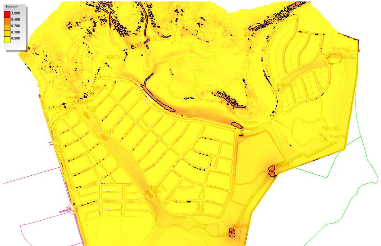
Figure E.15 – Flood Hazard Mapping Across the Developed Riverside Site – 6hr 100yr Storm, Extreme Tailwater (VxD=0.4 contour highlighted)
