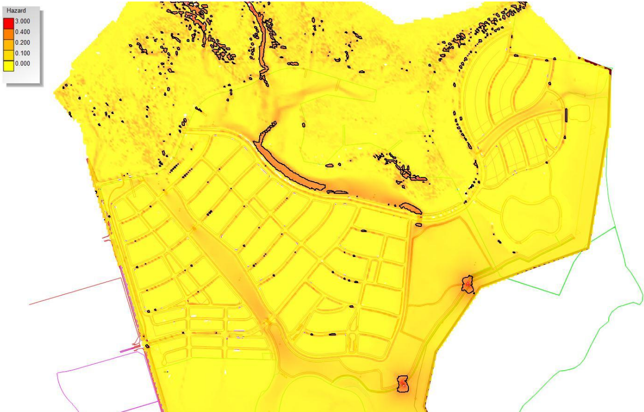
Figure E.13 – Flood Hazard Mapping Across the Developed Riverside Site – 3hr 100yr Storm, Extreme Tailwater (VxD=0.4 contour highlighted)
