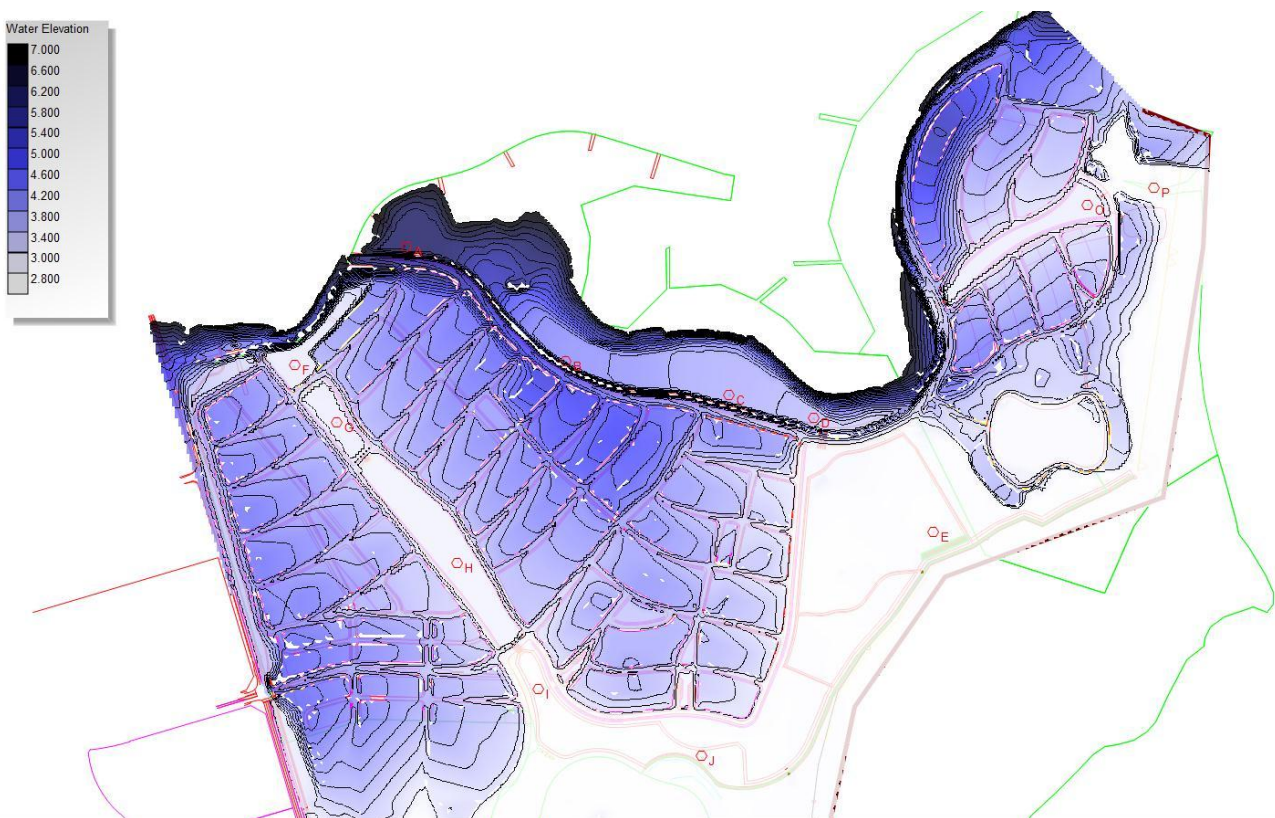
Figure 35 – Flood Level Contours Across the Developed Riverside Site – Event 2 Critical 2hr Storm – 5yr Storm, 2100 100yr Tailwater
