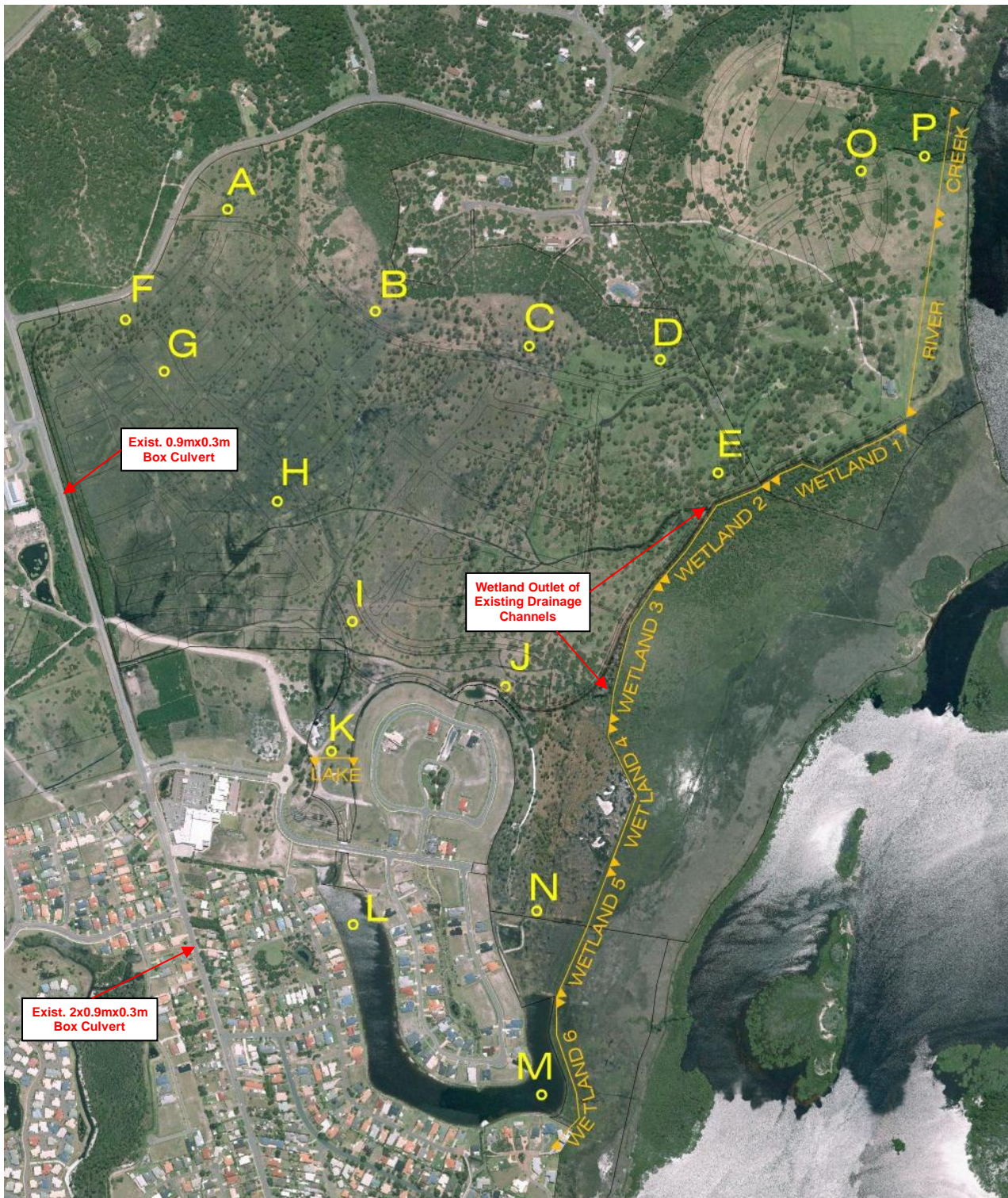
Figure 10 – Head/Velocity Sample Points and Flow Lines
