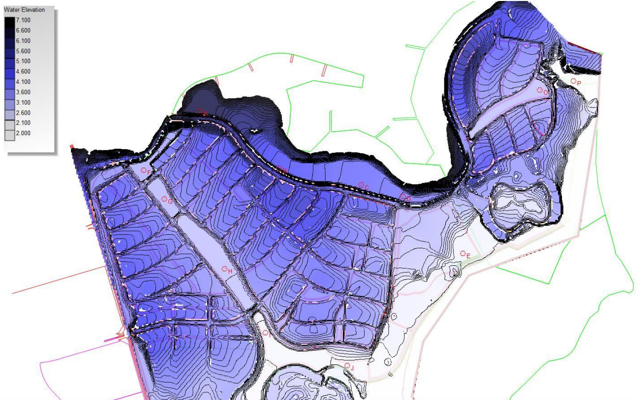
Figure 33 – Flood Level Contours Across the Developed Riverside Site – Event 1 Critical 2hr Storm – 100yr Storm, 2100 5yr Tailwater
