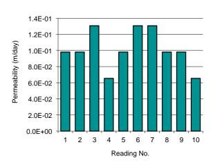
Note: Permeability  $K = 4.4Q\{\sinh^{-1}(H/2r)-[(r/H)^2+0.25]^{0.5}+(r/H)\}/2piH^2$  where Q = infiltration rate, H = depth of water in test hole, r = hole radius and pi = 3.1416. H should be in the range 5r to 10r. See Australian/New Zealand Standard 1547: 2000 On-site domestic-wastewater management. Appendix 4.1F.
