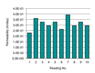
Note: Permeability K = 4.4Q{sinh<sup>-1</sup>(H/2r)-[(r/H)<sup>2</sup>+0.25]<sup>0.5</sup>+(r/H)}/2piH<sup>2</sup> where Q = infiltration rate, H = depth of water in test hole, r = hole radius and pi = 3.1416. H should be in the range 5r to 10r. See Australian/New Zealand Standard 1547: 2000 On-site domestic-wastewater management. Appendix 4.1F.
