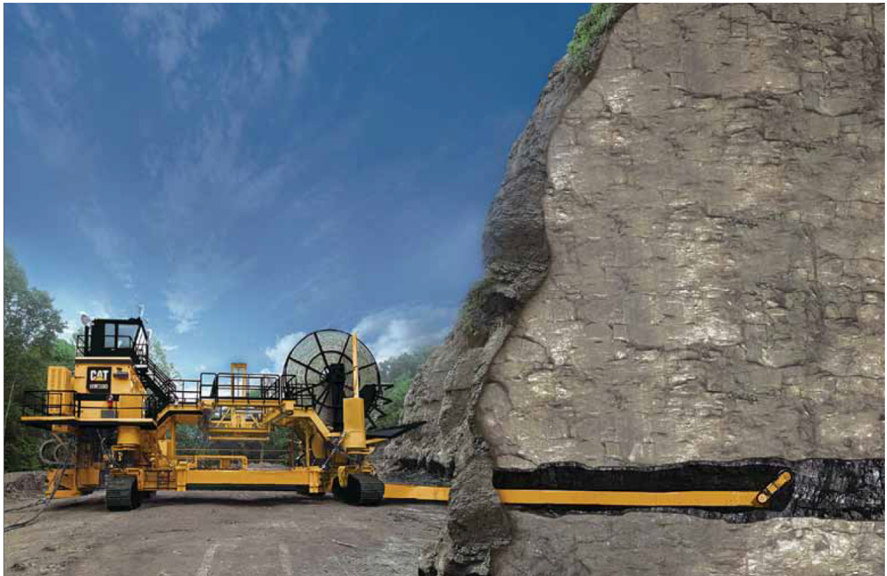
Figure 7. Typical HWM equipment and mine cross-section ( source: Coalpac )
