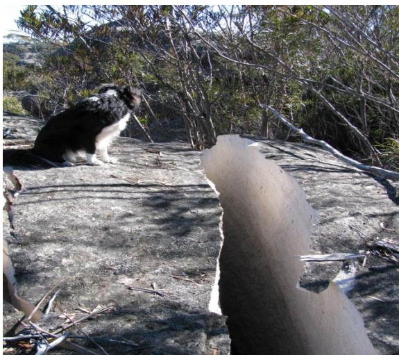
Crack & Cliff Fall: Baal Bone LW 28, July 2009 – the SMP only monitors damage, it doesn't prevent it.
