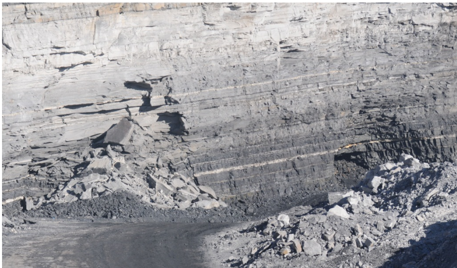
Figure 5 View of highwall intersecting old coal mine workings.
