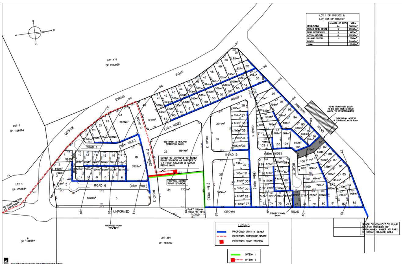
Figure 3.3: Proposed Sewerage Services
