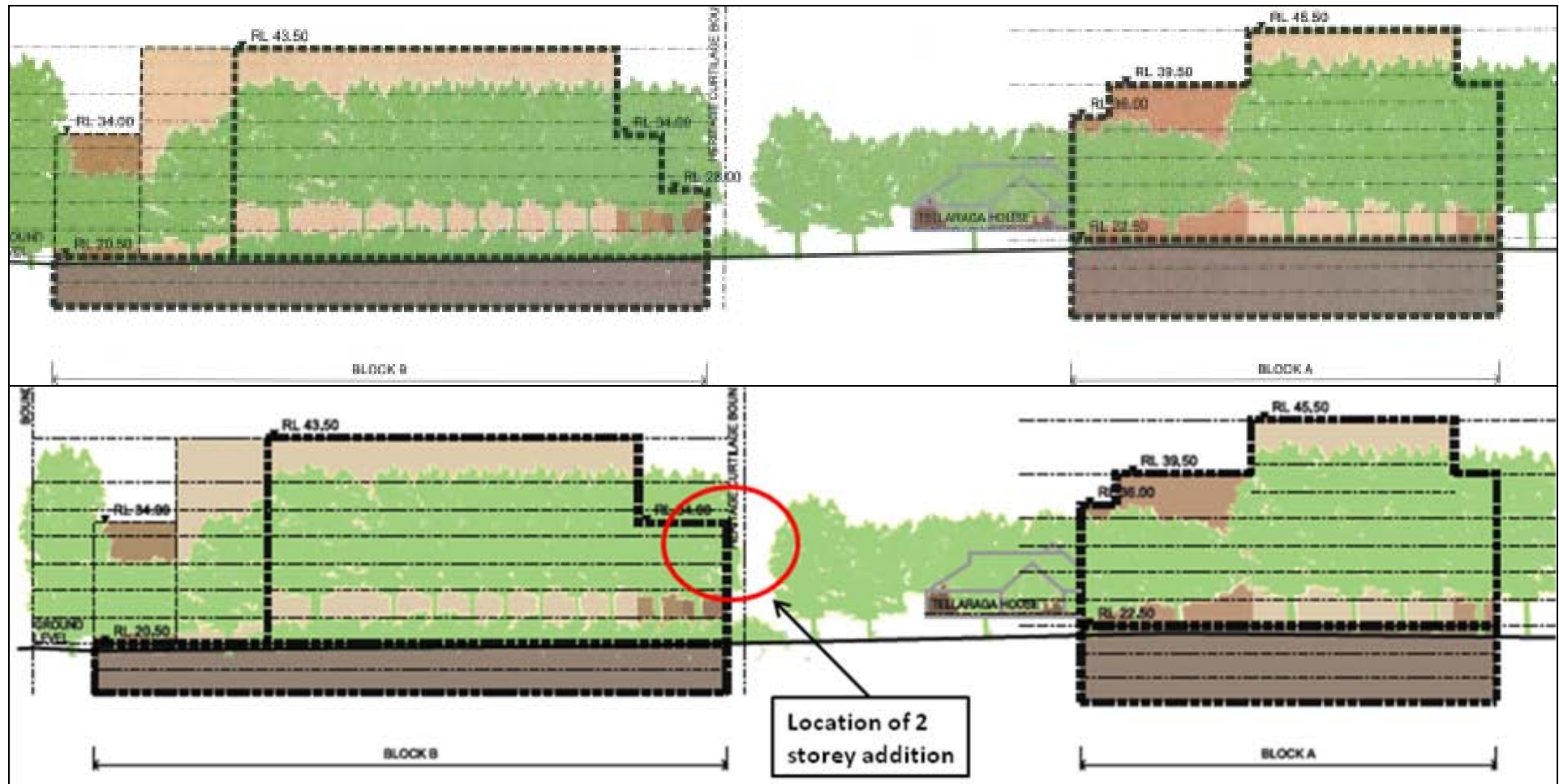
Figure 5: Comparison of the building envelope of Building B (western elevation as seen from Belmore Street): approved (above) and modified (below) (Source: Proponent's Environmental Assessment and original approval MP10_0110)
