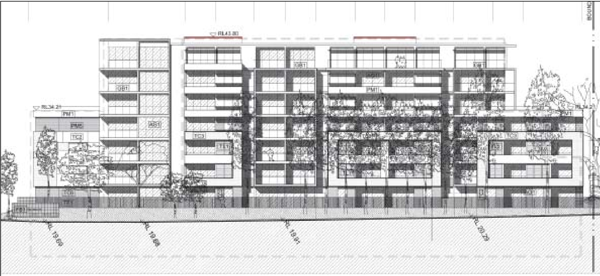
Figure 6: Increase of lift overrun by 300mm to Building B (Source: Proponent's Environmental Assessment)
