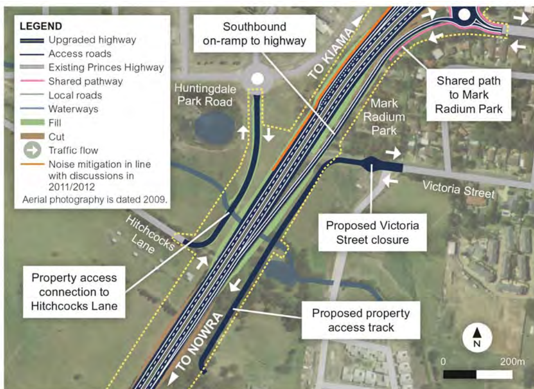
Figure 3.9 Victoria Street access arrangement
