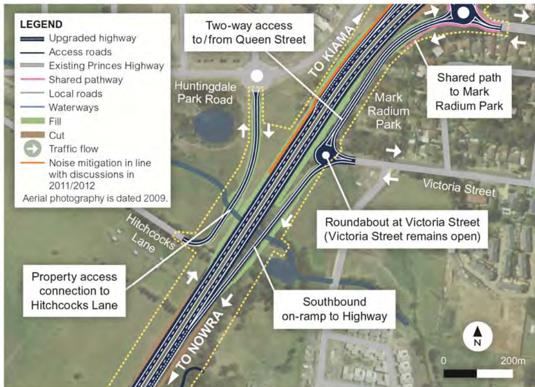
Figure 3.10 Victoria Street access arrangement
