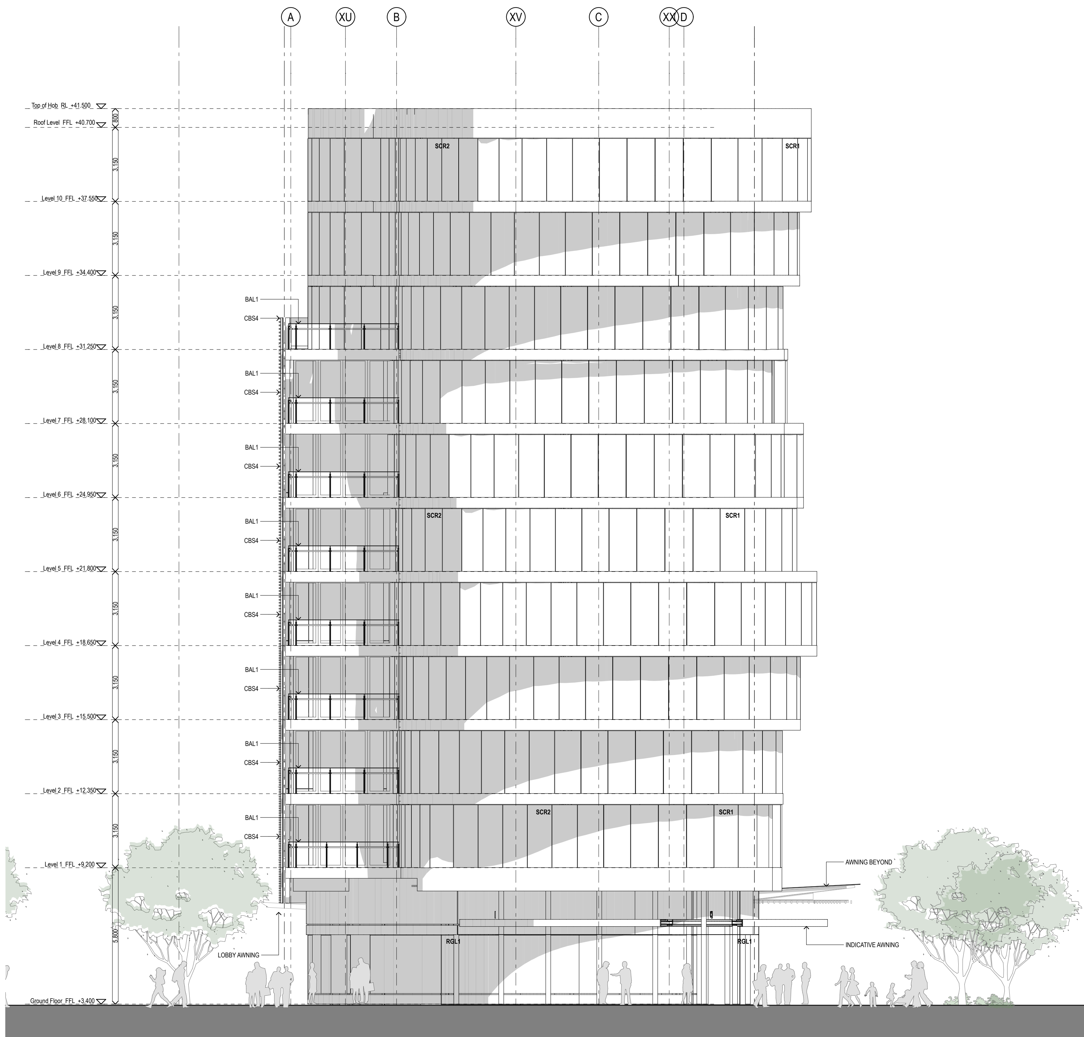
1 ELEVATION North Elevation 1:100
