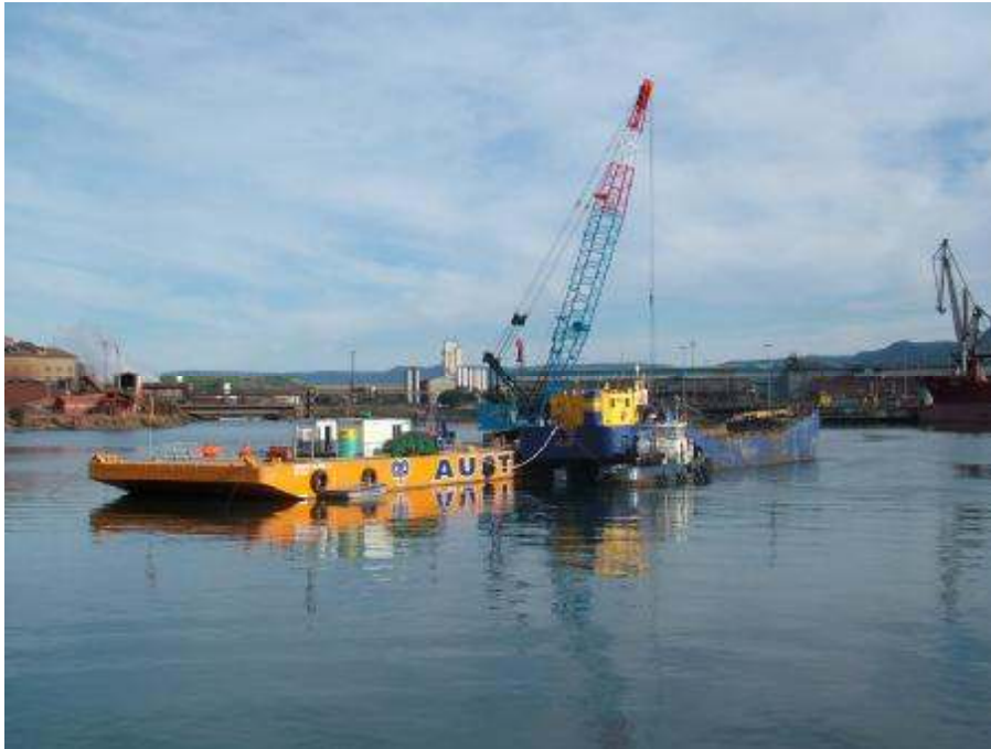
Photo 3.1 Grab dredger loading a self-propelled hopper barge
