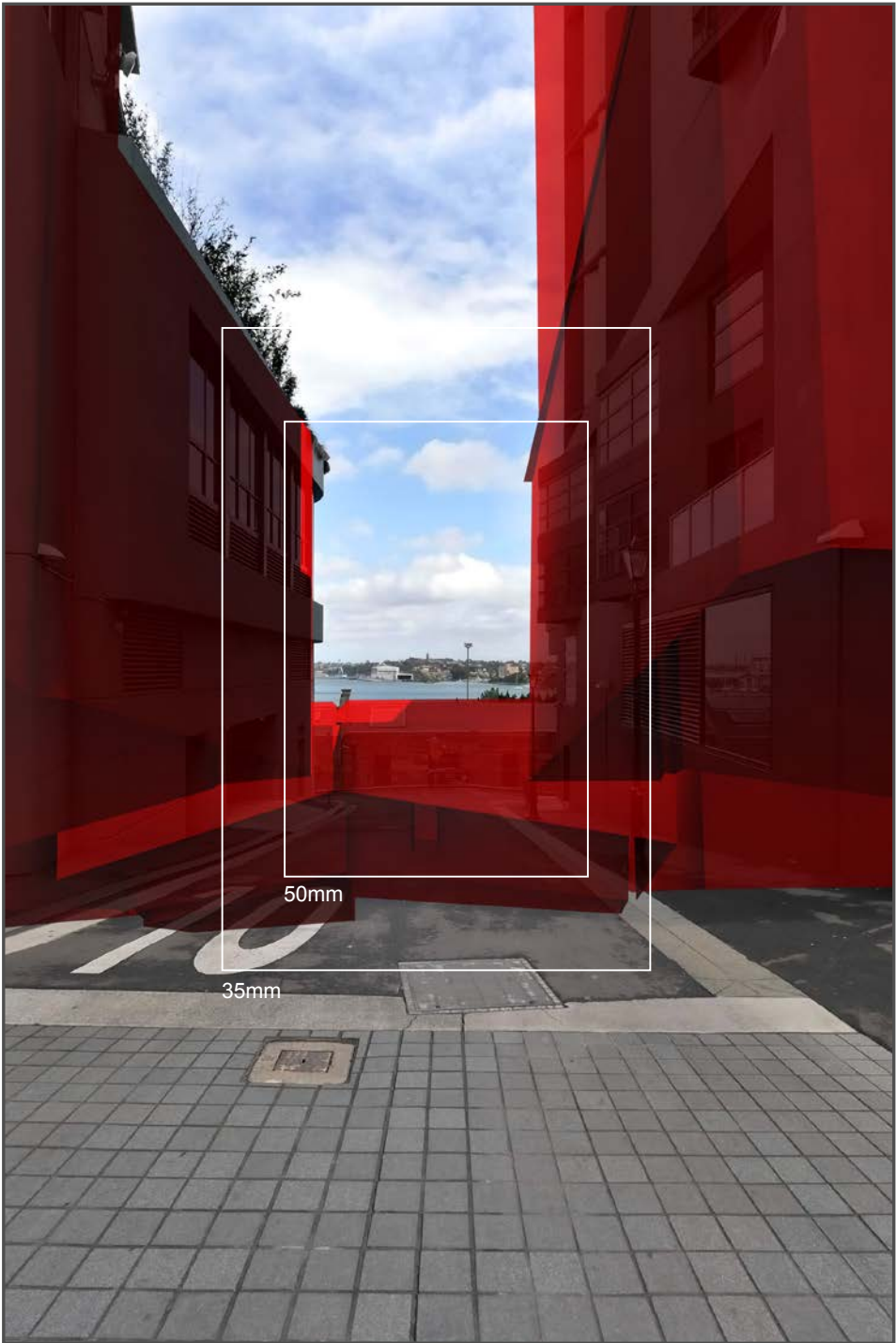
Image showing alignment of 3D model to photograph with the 3D model shown over in red.
