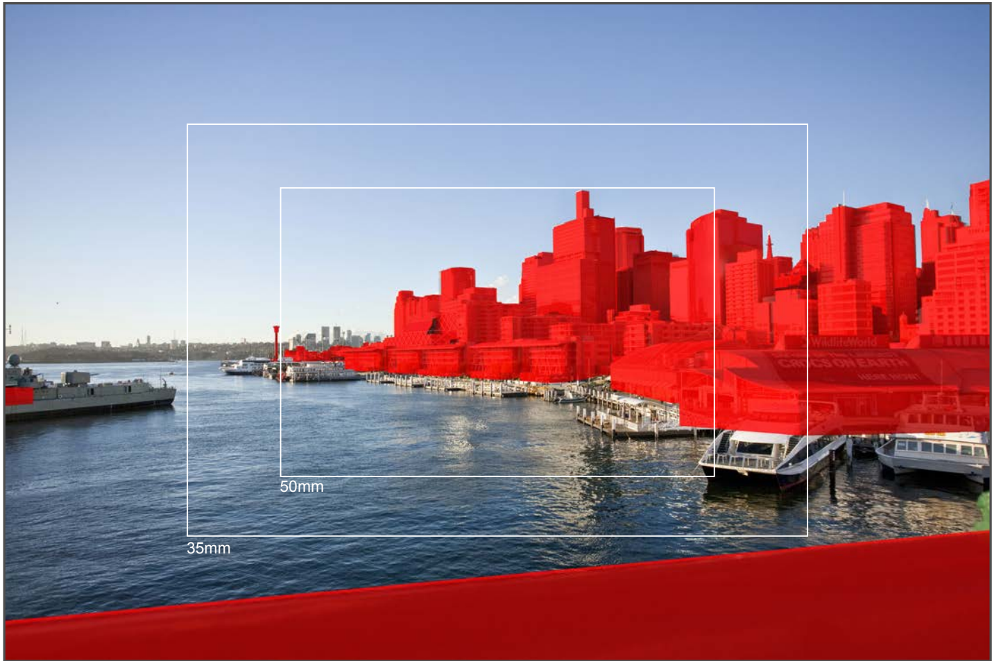
Image showing alignment of 3D model to photograph with the 3D model shown over in red.
