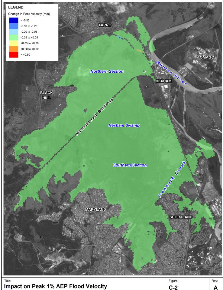
Impact on Peak 1% AEP Flood Velocity **Local Catchment Flood Conditions**
