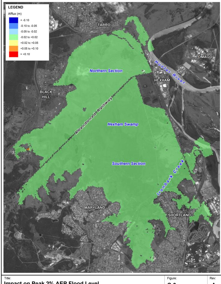
Impact on Peak 2% AEP Flood Level Local Catchment Flood Conditions
