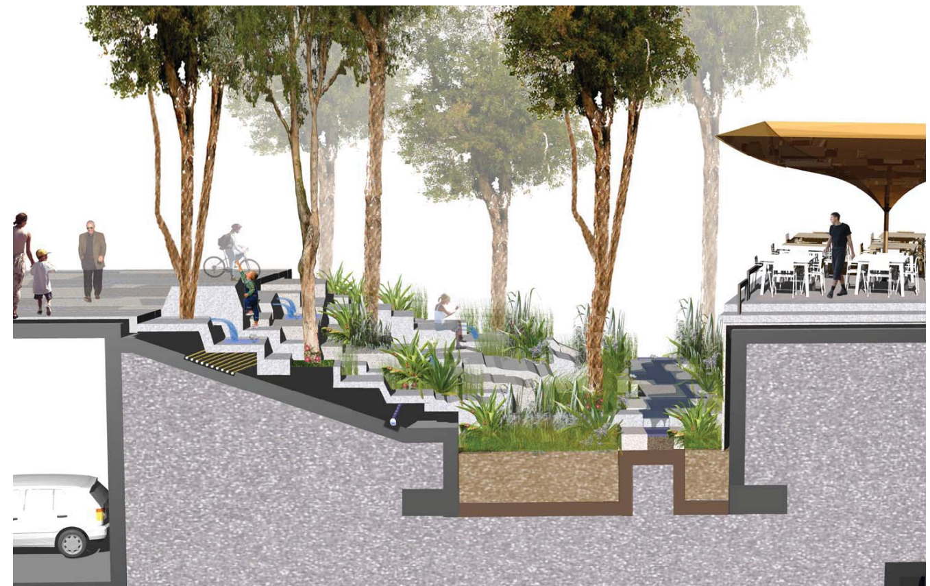
Below: Section diagram showing potential riparian park / plaza with integrated stormwater filtration and detention.
