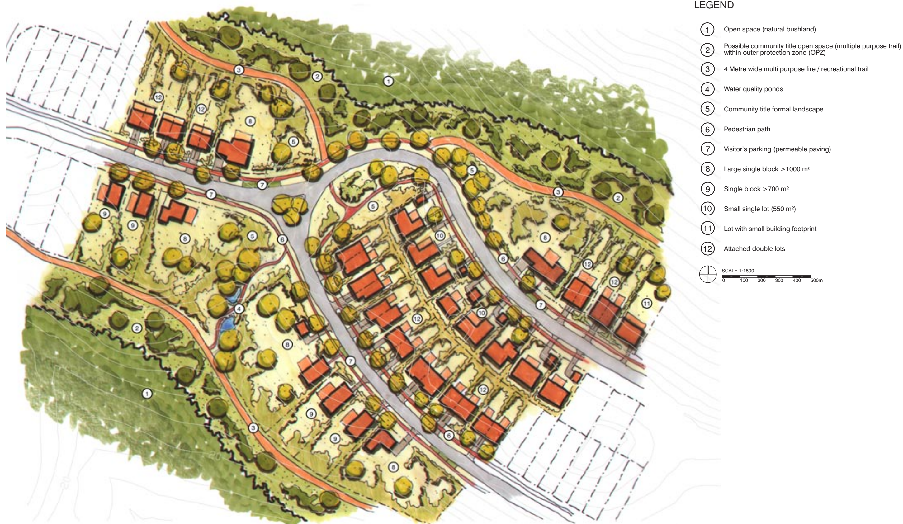
Figure 13: Partial plan showing different lot groups and the interaction between open spaces and asset protection zones
