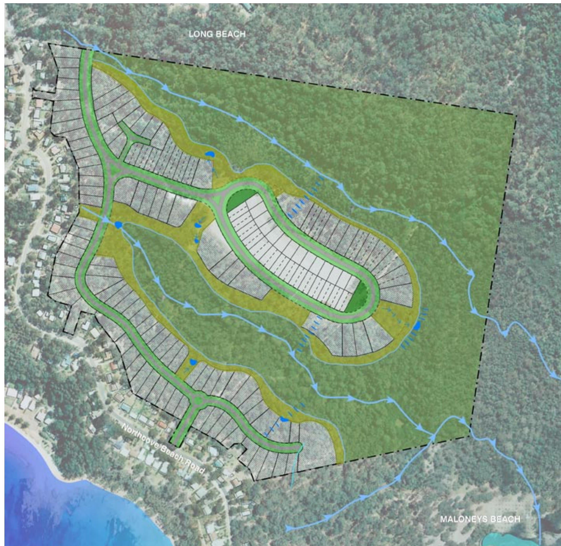
Figure 10: Lot layout with integrated open space and drainage network
