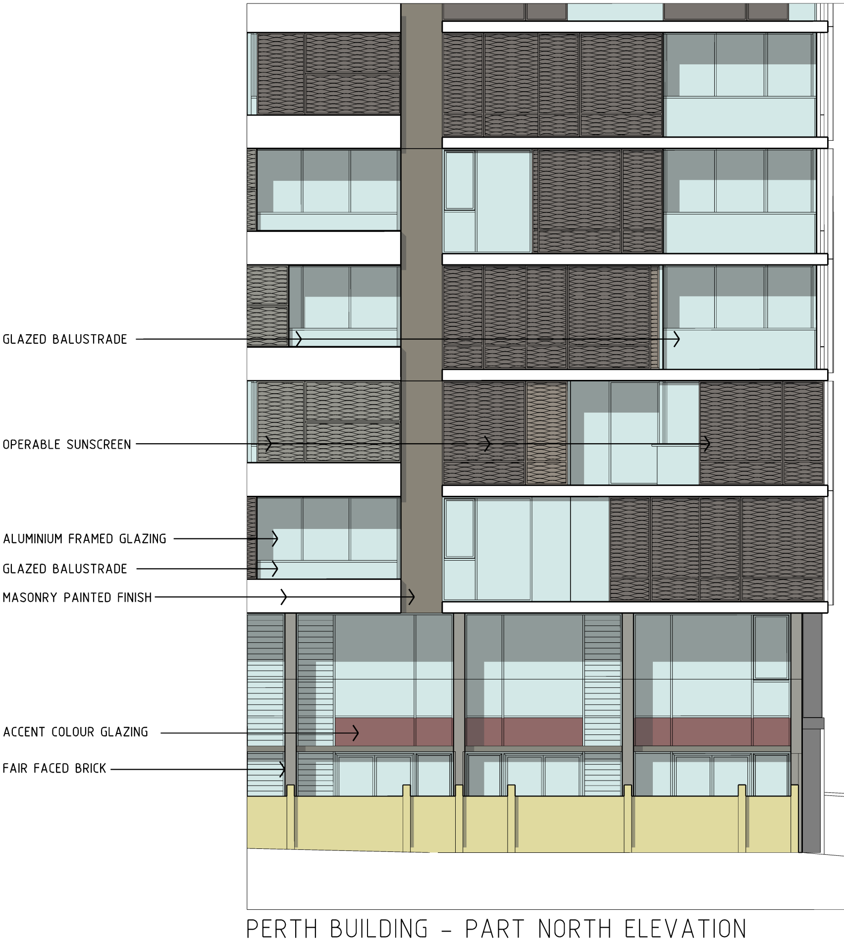
PERTH BUILDING - PART NORTH ELEVATION
