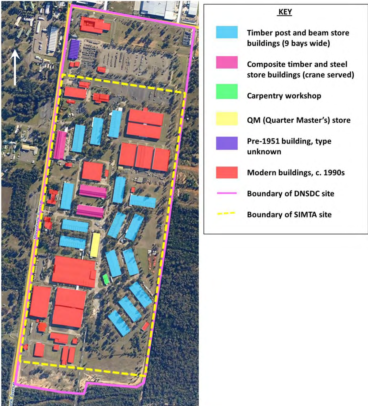
Figure 15: Plan showing the current location of building types within the DSNSDC site.
