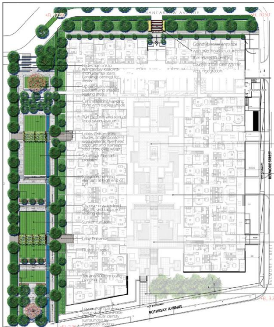
Figure 12: Extract of the Proposed Revised Foreshore Link Landscape Plan indicating the proposed foreshore link which now provides a more efficient access connection and introduces level pockets of passive recreation areas. This design improves the relationship of the foreshore link and the adjoining dwellings.
