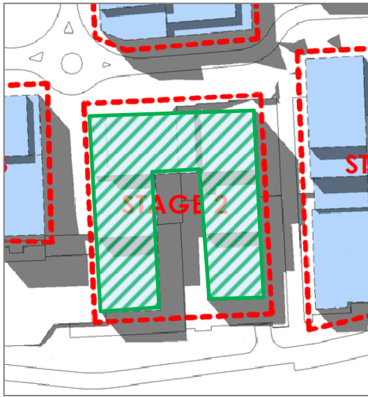
Figure 16: Demonstration of the basement parking level which is wholly contained within the building footprint.
