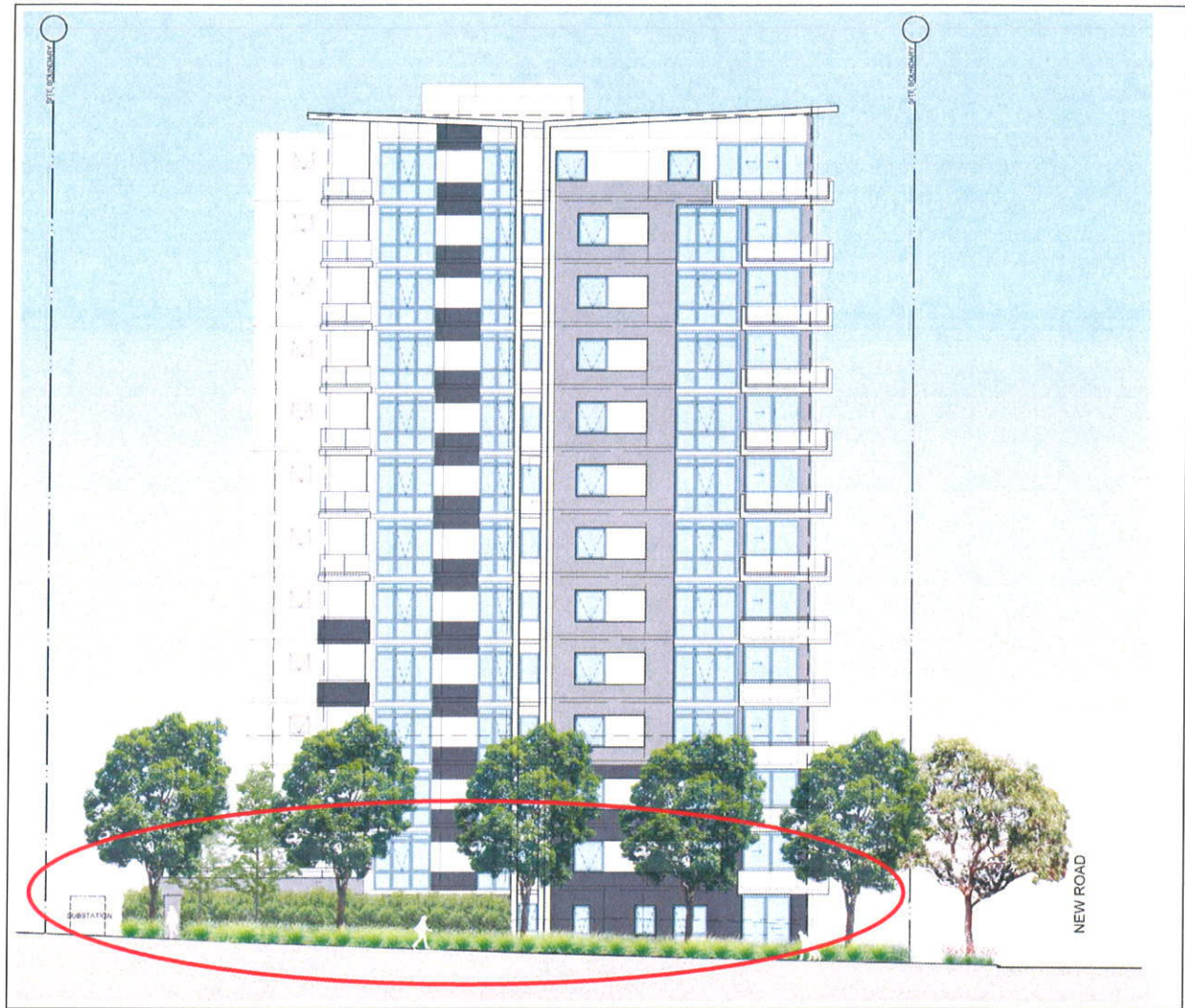
Figure 10: Proposed South East Elevation to Herring Road, showing additional landscaping to compensate for the removal of the mound.
