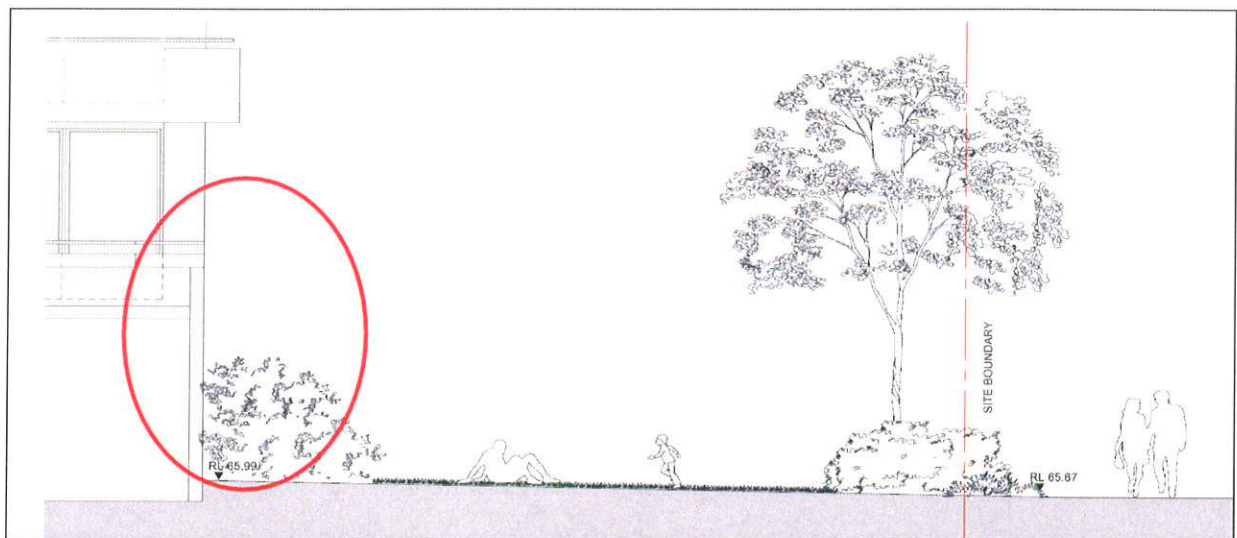
Figure 11: Detail Section of the proposed elevation to Herring Road, showing additional landscaping to compensate for the removal of the mound. The landscaping within the red oval is 'screening' a 3-4 metres high blank expanse of wall.
