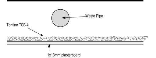
Pipework must be a minimum of 10mm from any support element or plasterboard
