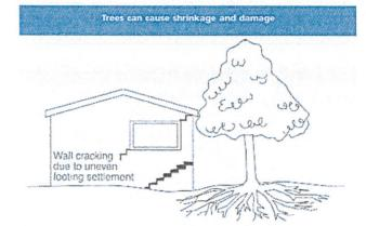
As the weather pattern changes and the soil begins to dry out, the external footings will be first affected, beginning with the locations where the sun's effect is strongest. This has the effect of lowering the external footings. The doming is accentuated and cracking reduces or disappears where it occurred because of dishing, but other cracks open up. The roof lines may become convex.
