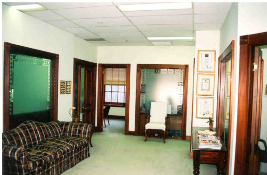
Figure 3-26 View of the fourth level office space, looking east, towards the George Street frontage. This level features painted light-weight partitions, suspended ceilings, carpeted floor and glazed timber internal doors
