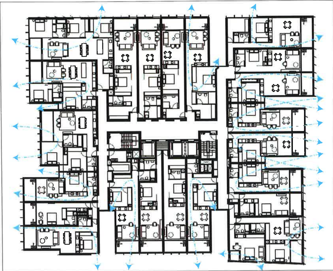
Figure 14: Typical cross flow ventilation (Source: Applicant's Rts)
