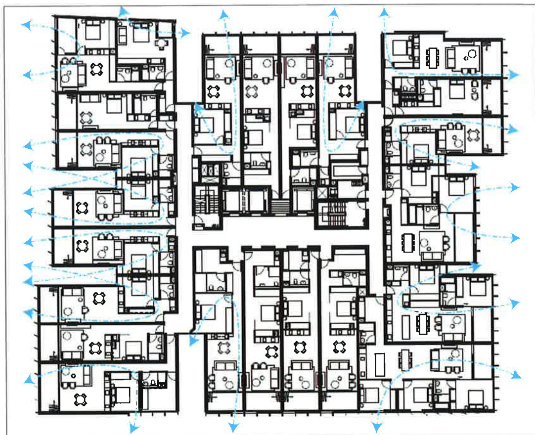
Figure 14: Typical cross flow ventilation (Source: Applicant's RtS)
