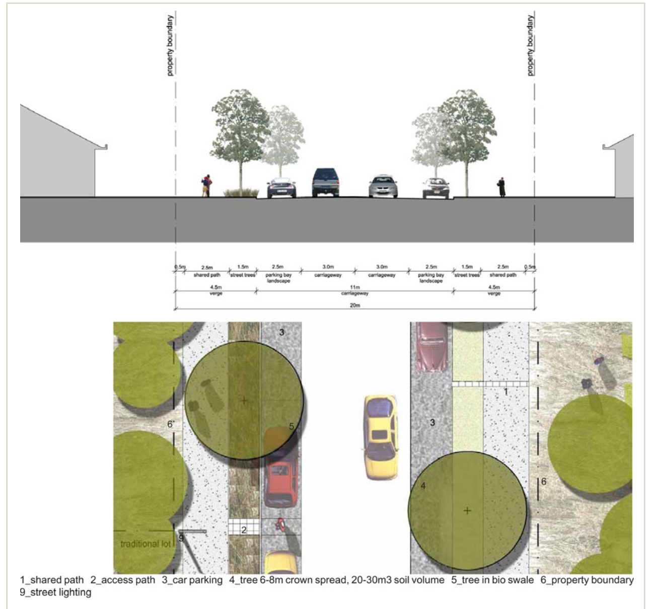
Figure B.1.13 Collector Road B - 20m (Section 4-4)
