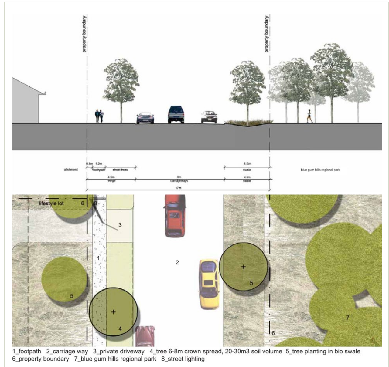
Figure B.1.15 Local Road A - 17m (Section 6-6)
