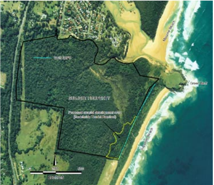
The shows the 2105 Zone of Reduced Foundation Capacity (ZRFC) at the subject property. Given that this line is just seaward of the property, there are no particular foundation requirements (from a coastal engineering perspective) for any structures built on the property in the next 100 years. However, there may be geotechnical issues to consider.
