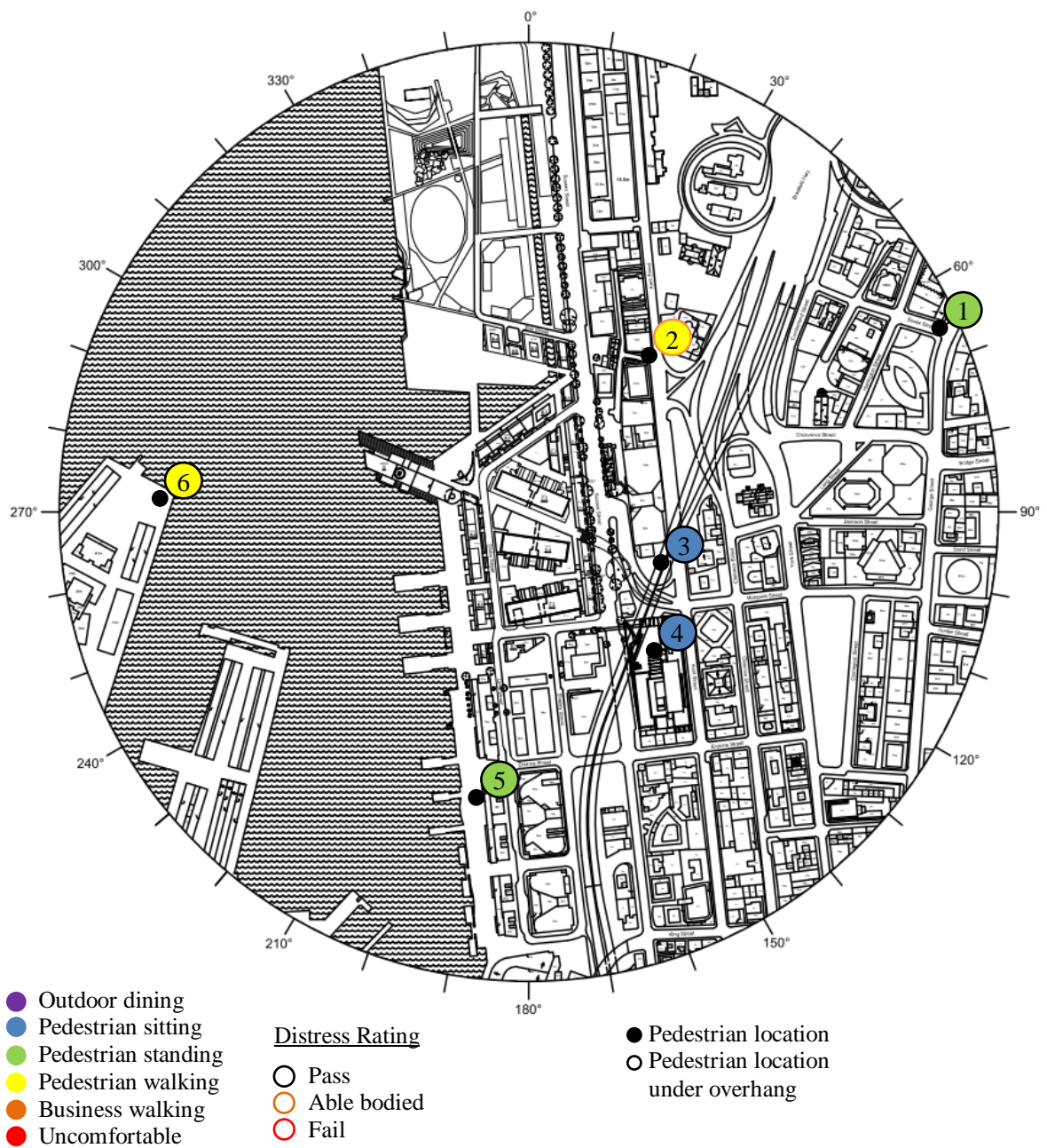
Figure 6: Remote pedestrian wind speed measurement locations with comfort/distress ratings
