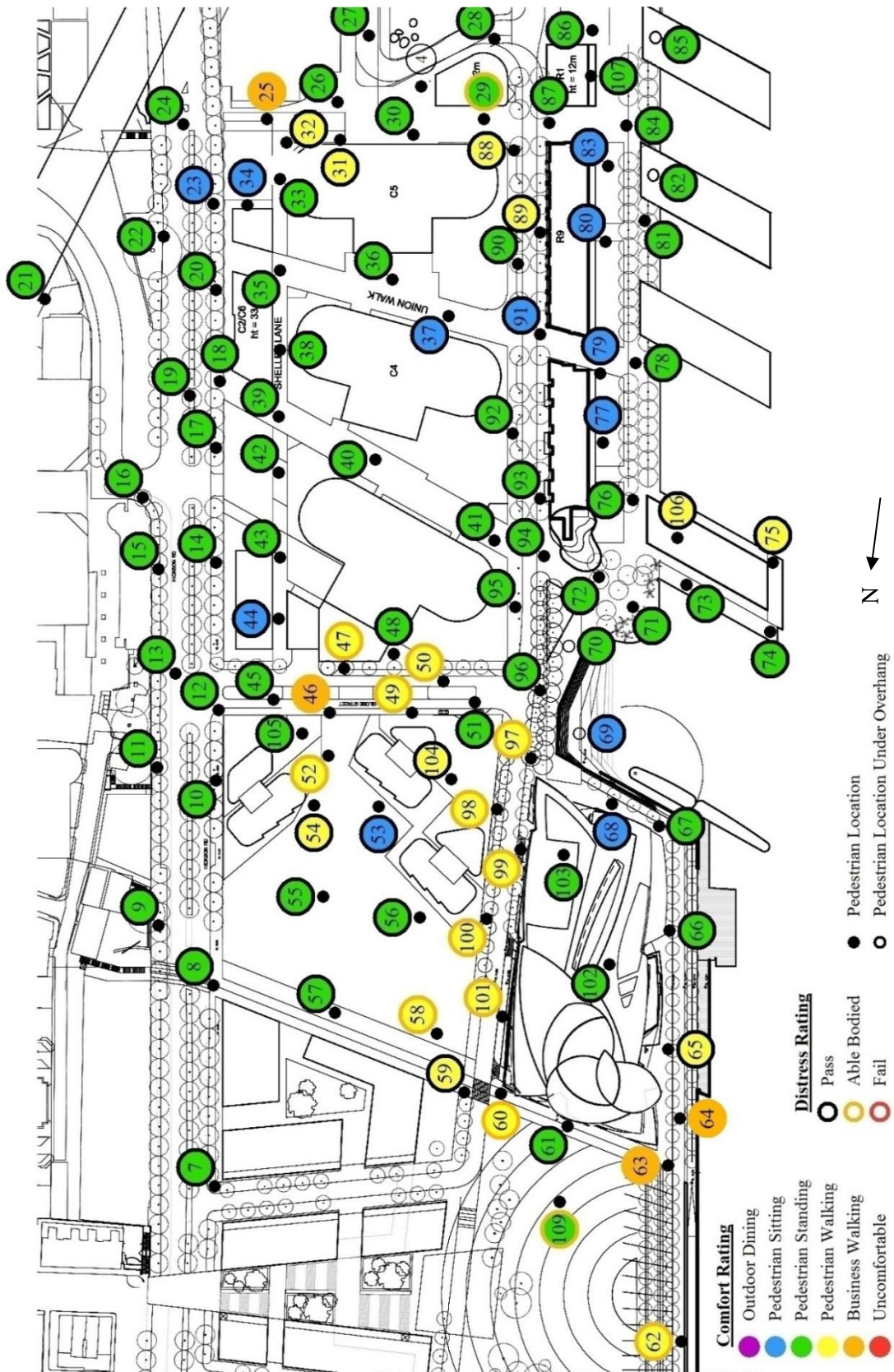
Figure 12: Pedestrian wind speed measurement locations – winter
