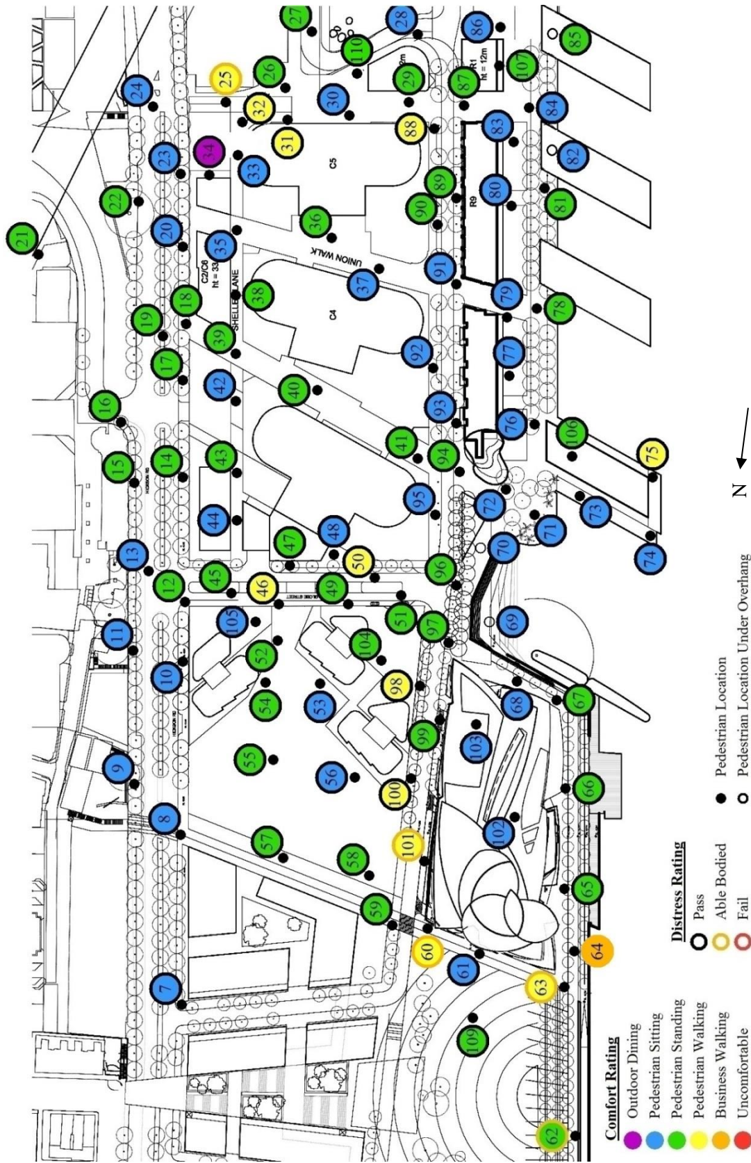
Figure 11: Pedestrian wind speed measurement locations – autumn
