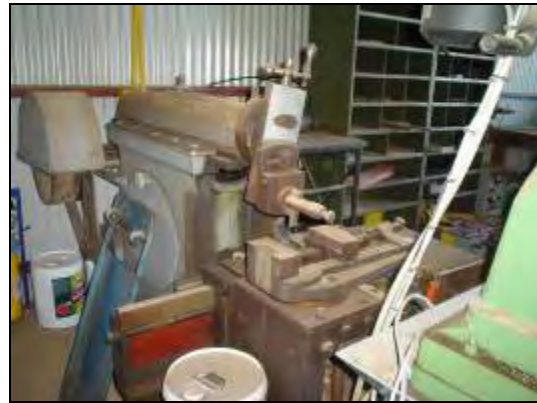
Figure 29 B – Wood shaper (c1940s)
