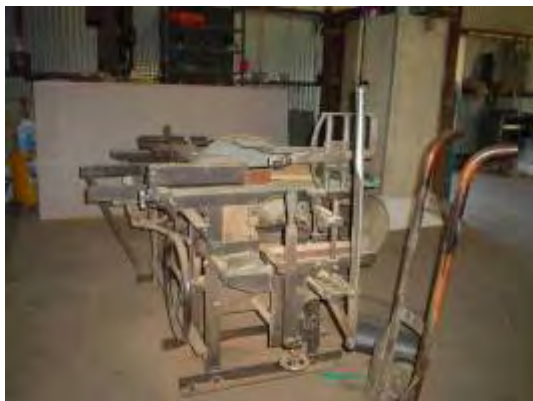
Figure 32 E – Combination saw/plane (early 1950s)
