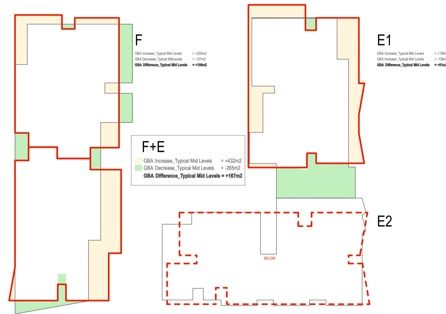
PROPOSED FLOOR PLATE COMPARISON TO INDICATIVE CONCEPT PLAN TYPICAL LOWER FLOOR LEVELS 1 - 6
