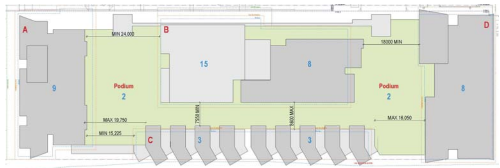
Figure 9 – Building separation distances
