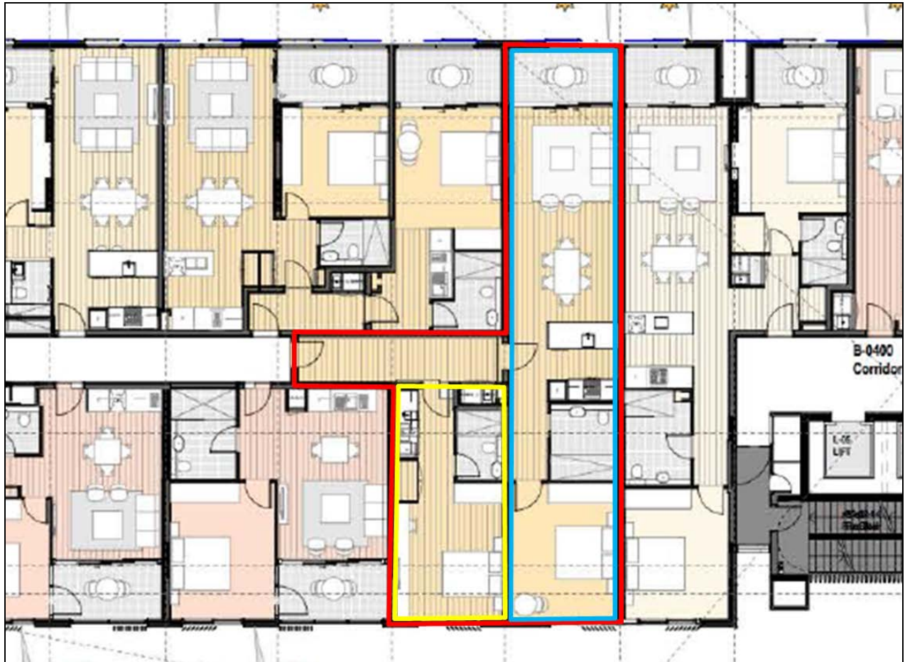
Figure 13: A dual key apartment (outlined in red) and the internal division between the studio and one bedroom apartments within (outlined in yellow and blue) (Source: applicant's RtS)
