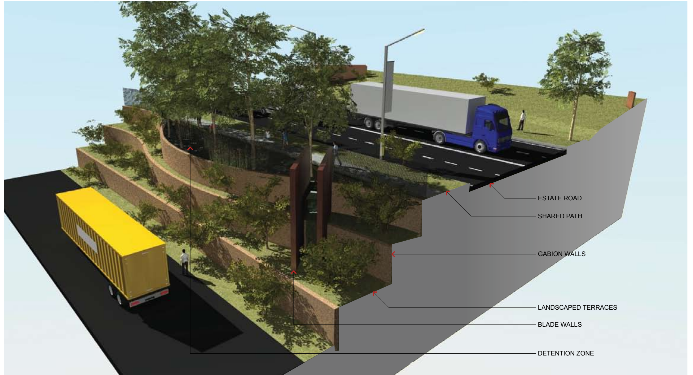
DETAIL SECTION OF RETAINING WALL SECTION A
