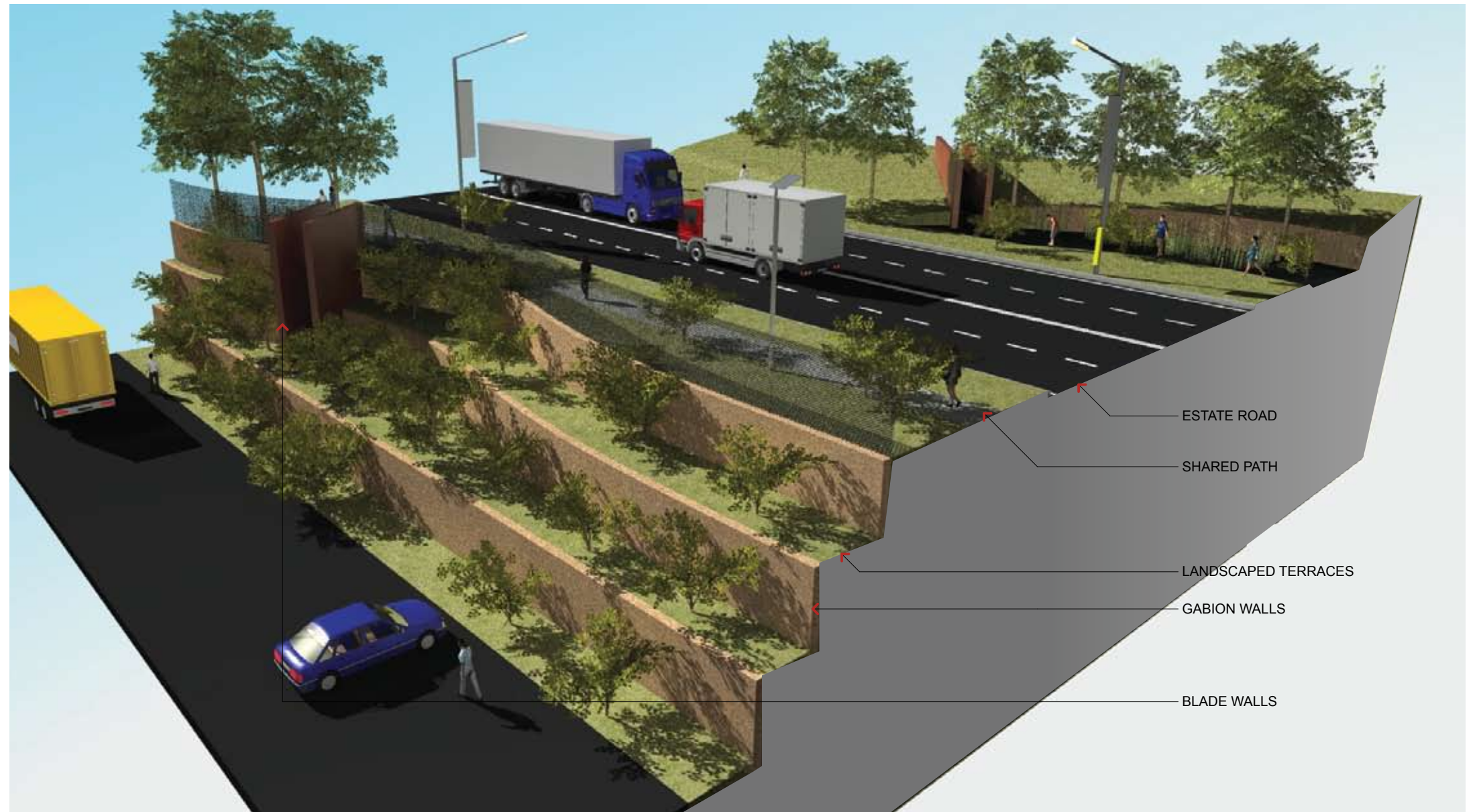
DETAIL SECTION OF RETAINING WALL SECTION B
