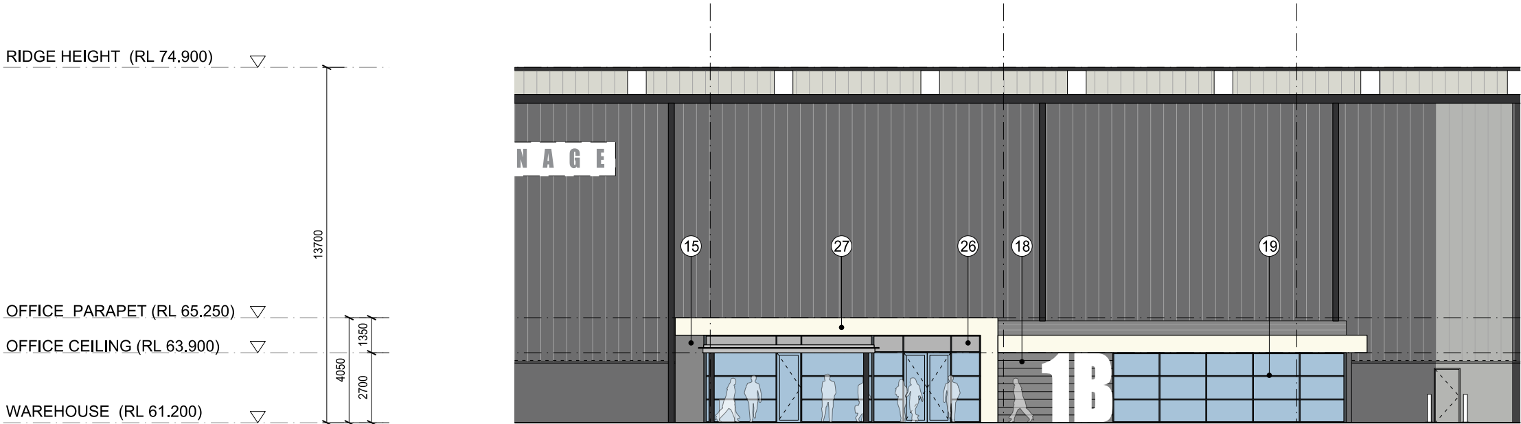
01 WEST ELEVATION OFFICE 2 - SCALE 1:200 @ A3
