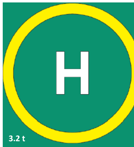
Figure C5: Example HLS with tonnage marking (in this case up to 3.2 tonne static load).
