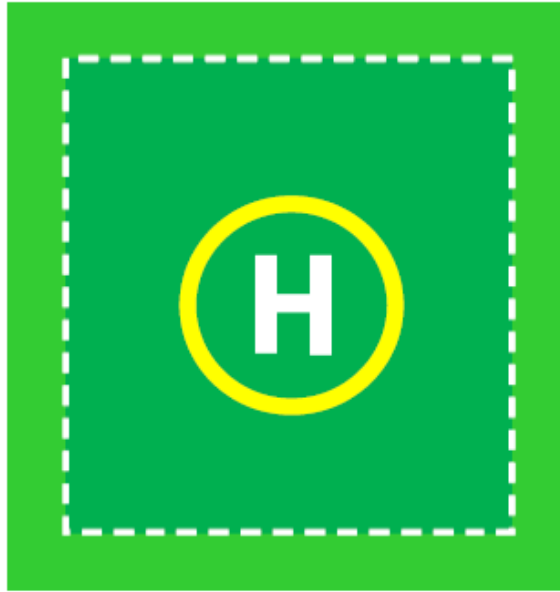
Figure C3: Secondary HLS: A 1.5 \times D FATO with additional 0.25 \times D Safety Area (Total area is 2 \times D ). Also showing 'H', FATO perimeter and 0.5 \times D Touchdown/Positioning Markings (TD/PM).
